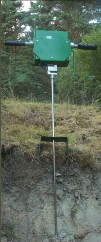
Fig.2: Rimik CP20 Cone Penetrometer
