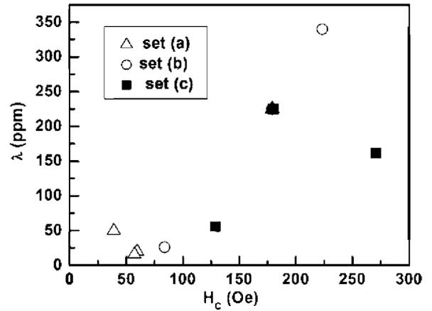
Fig. 3. Magnetostriction constant as a function of the coercivity for the three set of samples: set (a) (△), set (b) (○), and set c (■). We have not included in the graph those samples with a coercivity higher than 275 Oe.
