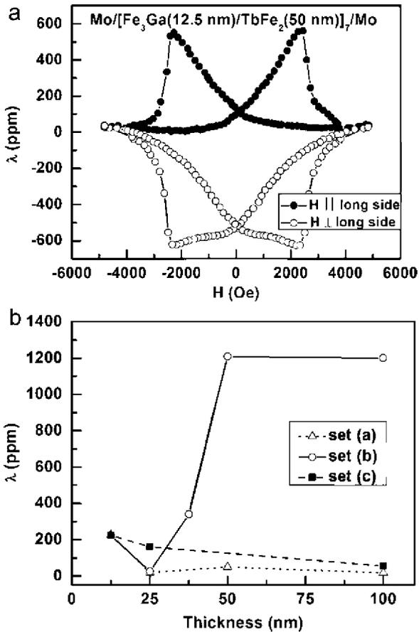
Fig. 2. (a) Magnetostriction as a function of the applied magnetic field of the [Fe<sub>3</sub>Ga(12.5 nm)/TbFe<sub>2</sub>(50 nm)]<sub>7</sub>. The direction of the magnetic field is parallel (●) and perpendicular (○) to the long side of the cantilever. (b) Magnetostriction constant as a function of the thickness layer for the three set of samples: set (a) (△), set (b) (○), and set c (■).
