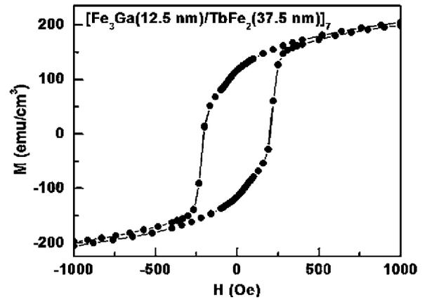
Fig. 4. Hysteresis loop at room temperature of the [Fe<sub>3</sub>Ga(12.5 nm)/TbFe<sub>2</sub>(37.5 nm)]<sub>7</sub> heterostructure.
