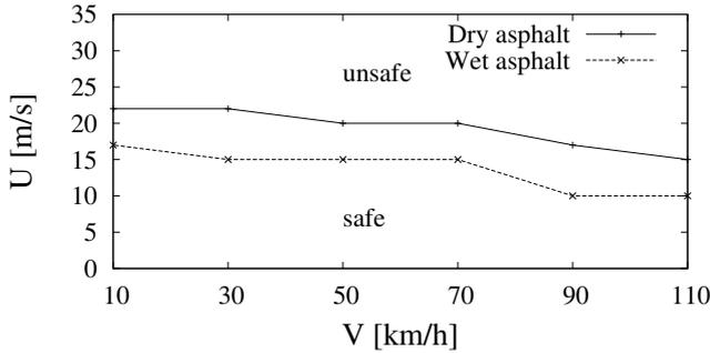
Figure 6. CWC in a rigid road without roughness.
