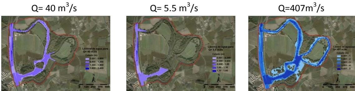
Figure 2-. Depth of water after hydraulic simulation in two different restoration alternatives for the meanders of Ramalhondo and Soto Gil (River Arga)
