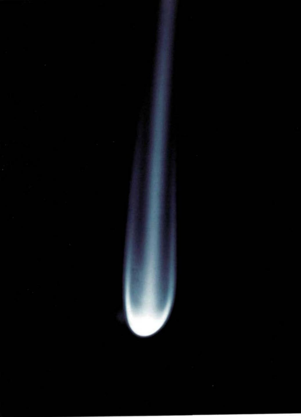
Fig. 1. Typical photograph of a stationary triple flame in a coflowing stream stabilized in the burner described herein. Details can be found in subsections 2.1 and 2.2.
