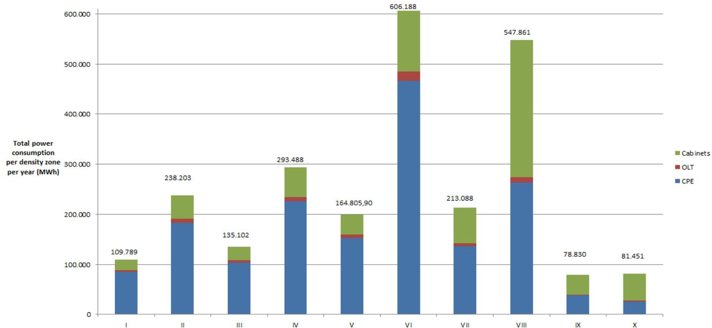
Total power consumption per density zone (MWh) of the FTTx/VDSL architecture and participation of each network active element.
