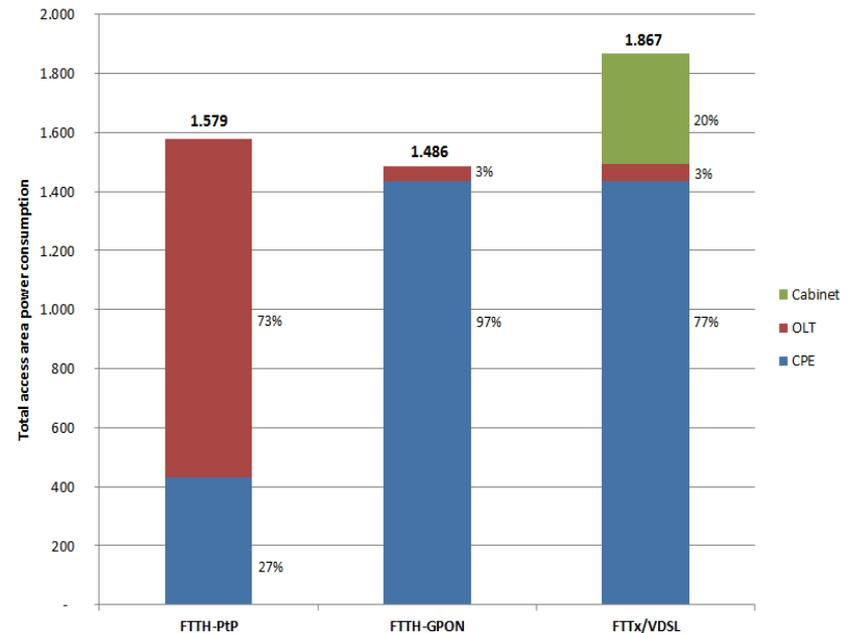
Percentage of power consumption for each active element of the fibre-based networks vs. the total power consumption in the access area (according to the sizing for density zone VI).
