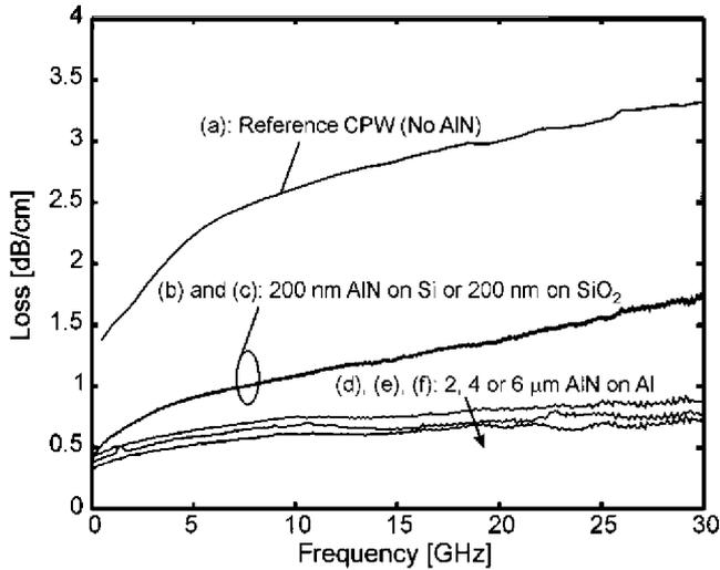
**Fig. 2.** Measured microwave losses for 5 different CPWs: (a) CPW on 330 nm  $\text{SiO}_2$ ; (b) CPW on 200 nm AlN deposited directly on the silicon substrate; (c) CPW on 200 nm AlN deposited on 30 nm  $\text{SiO}_2$ ; (d) 2  $\mu\text{m}$  AlN, (e) 4  $\mu\text{m}$  AlN, and (f) 6  $\mu\text{m}$  AlN deposited on a CPW as in (a).
