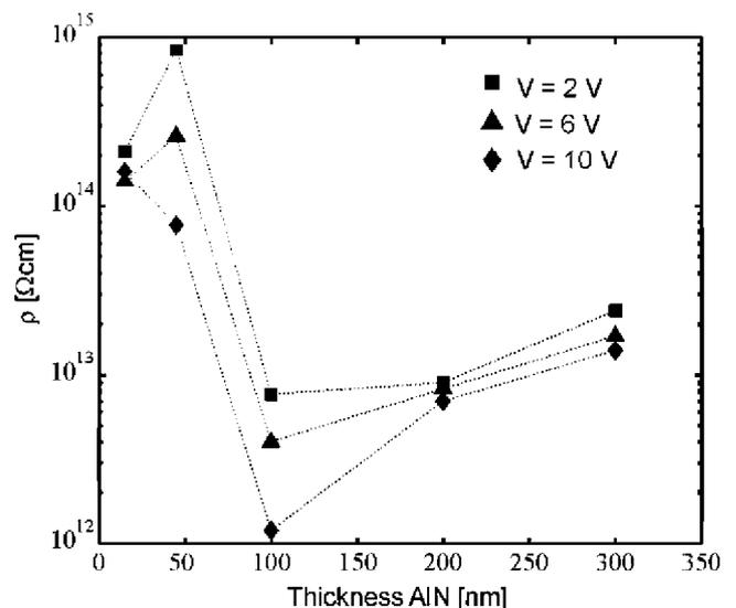
Fig. 1. Resistivity as a function of AlN thickness for different values of the voltage applied to the terminals of Al–AlN–Si capacitors.
