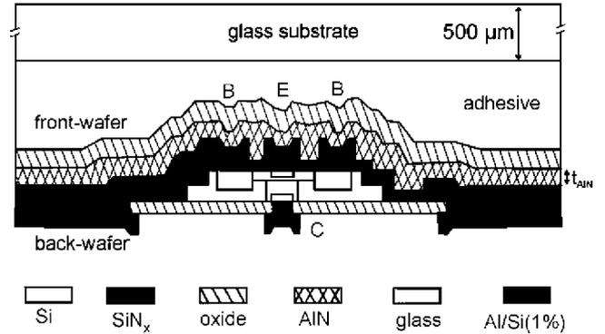
**Fig. 3.** Schematic cross-section of a silicon-on-glass bipolar junction transistor with an AlN layer deposited on the front-wafer.
