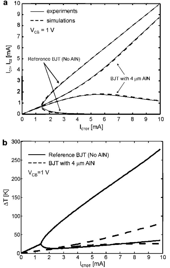
**Fig. 5.** (a) Measured (solid lines) and simulated (dashed lines) collector currents of the individual transistors of a pair operated in parallel as a function of the total collector current for the reference device and a device with a 4  $\mu\text{m}$ -thick layer of AlN. (b) Simulated increase of temperature above ambient of the individual transistors of a pair, without (solid line) or with (dashed lines) a 4  $\mu\text{m}$ -thick layer of AlN.
