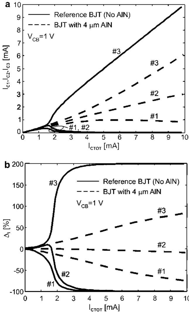
**Fig. 6.** (a) Measured collector currents of the individual transistors of a set of three operated in parallel as a function of the total collector current for the reference device (solid lines) and a device with a 4 μm-thick layer of AlN (dashed lines). (b) Discrepancy  $\Delta_i$  of the individual collector currents with respect to the thermally ideal situation versus  $I_{CTOT}$ .
