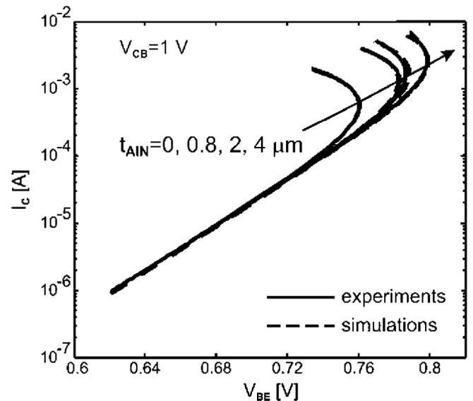
**Fig. 4.** Collector current as a function of the base-emitter voltage for an NPN covered with AlN layers of different thicknesses  $t_{\text{AlN}}$ .
