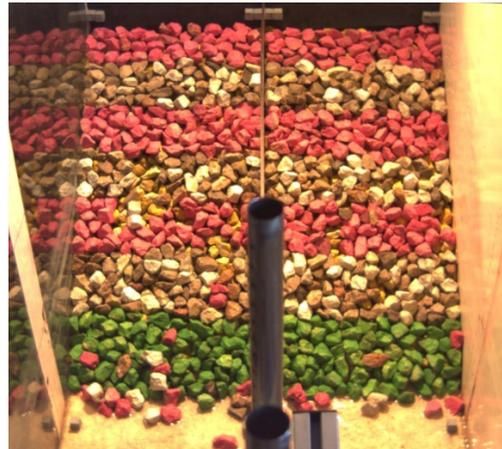
Figure 1 - Example of damage accumulation test at the HRL (Harbour Research Laboratory) of the Polytechnic University of Madrid.
