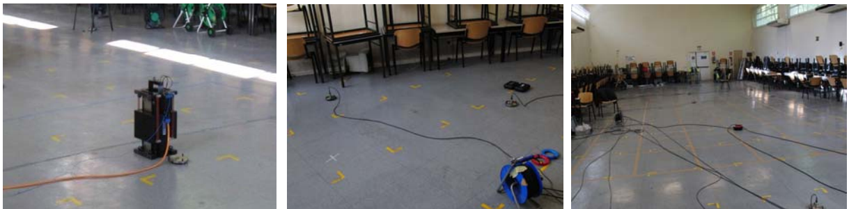
Figure 2. Shaker and accelerometer test layout and three photographs of the instrumentation .
