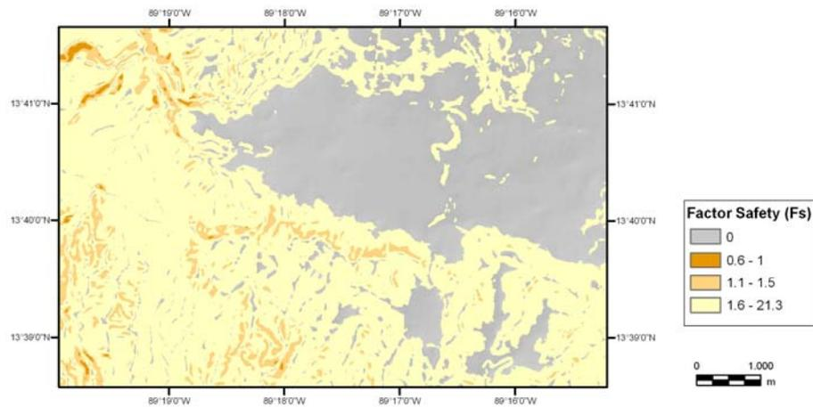
Figure 2 Factor safety (Fs) using the expression: with dry conditions
