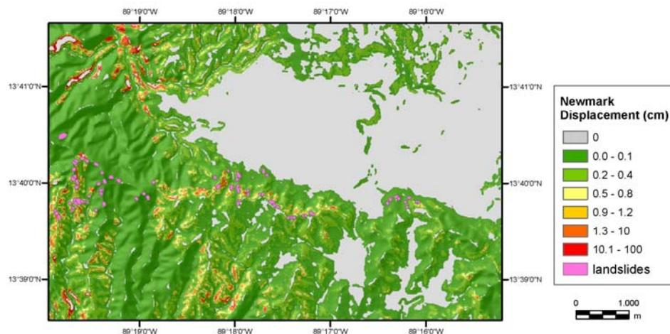
Figure 6 Newmark Displacement for the 13<sup>th</sup> January 2001 earthquake scenario in San Salvador, considering site effect, together the inventory landslides.
