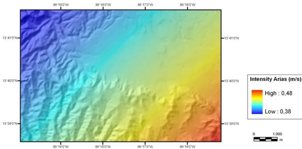
Figure 4 Estimated Arias intensity (g) in rock
