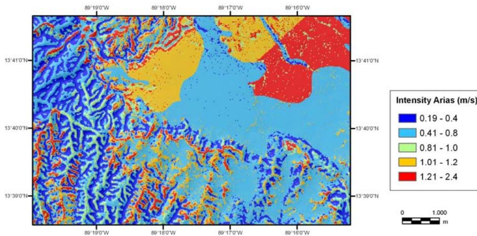
Figure 5 Estimated Arias Intensity ( $I_a$ ) with geology and topography amplification factor.
