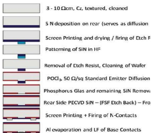
Figure 6 : Processing scheme of EWT cells
