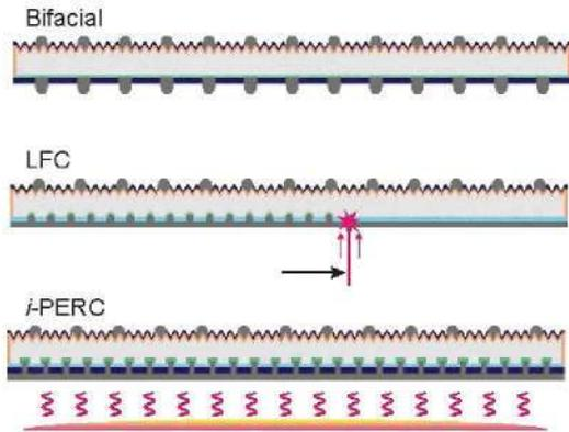
Figure 3 : The passivated rear surface solar cells on low cost substrates can be classified in three groups: bifacial solar cells with fire-through contacts, laser fired contact solar cells, and selective alloying, thermally fired LBSF solar cells (i-PERCs)
