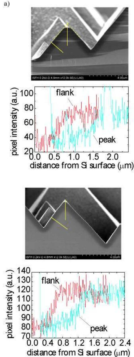
Figure 4 : Emitter profile measured by secondary electron SEM. Darker regions correspond to n-type silicon. a) spray-on in-line diffusion, b) POCl<sub>3</sub> sample. The profiles are in both case about 0.5-1 μm at the pyramid flank, and ~ 1-1.5 μm at the peaks.
