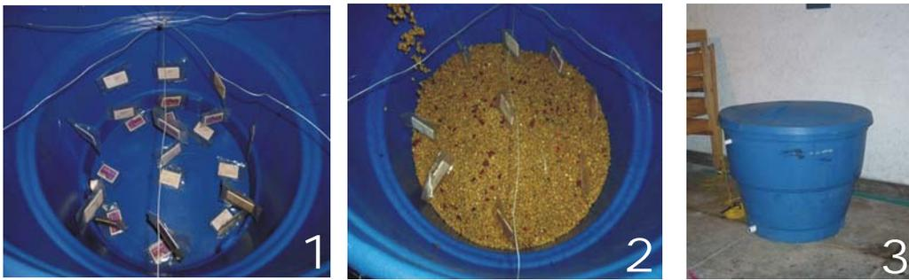
**Figure 1.** Images of experiment setup: 1. placement of sensors, 2. filling the tank, 3. fermentation.
