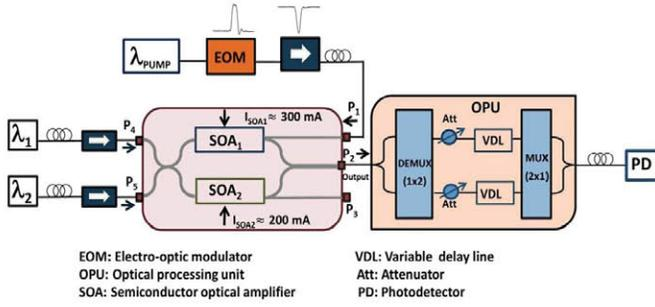
Fig. 1. Experimental design for UWB signal generation and customization.
