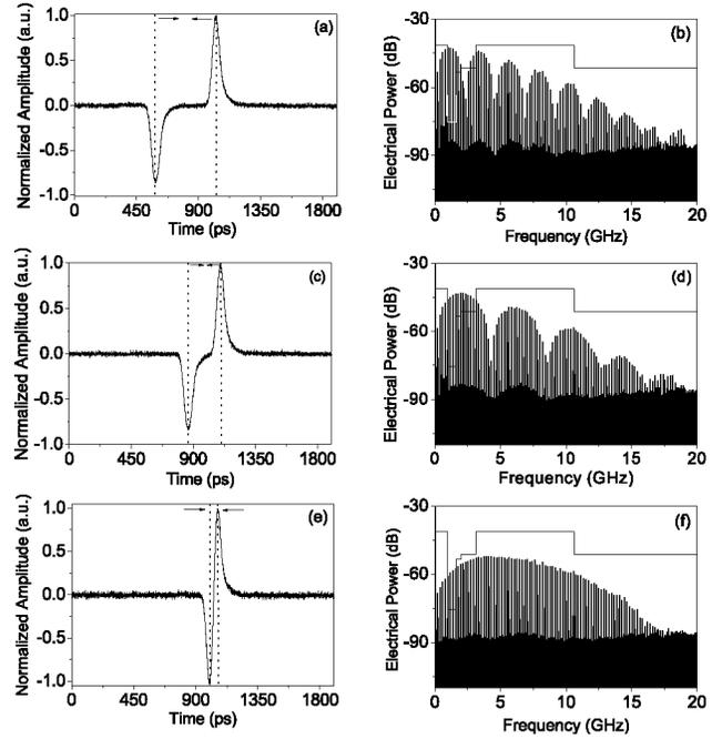
Fig. 5. (a) Generated pulses in their original position, prior to the delay configuration, (b) corresponding spectral representation, (c) generated pulses with a 200 picoseconds approximation, (d) spectral representation for the modified pulses, (e) obtained monocycle waveform after final delay configuration and (f) spectrum for the obtained UWB monocycle pulse.
