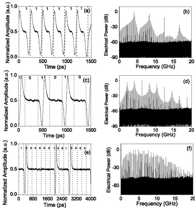
Fig. 6. (a) First data scheme transmitted with a bit sequence of all ones “1” and (b) corresponding spectral representation. (c) Second data series composed of both ones “1” and zeros “0” bits and (d) respective spectrum. (e) Third data sequence transmitted and (f) electrical spectrum.
