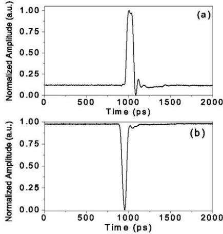
Fig. 2. (a) Electrical input pulsed signal prior to the EOM and (b) modulated optical pulse employed as pump signal.
