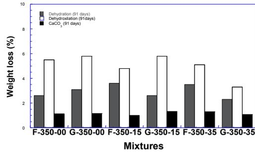
Fig. 10 – Thermogravimetry/Differential Thermal Analysis (91 days)
