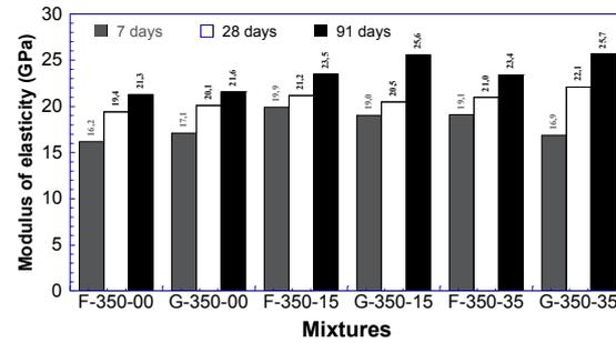
Fig. 3 – Modulus of Elasticity
