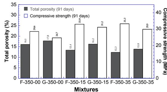
Fig. 5 – Compressive strength and MIP total porosity (91 days)
