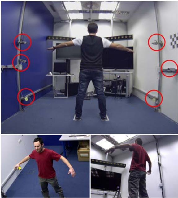
Figure 1: Typical camera setup. Top: a photo taken by one of the cameras of the setup, with other cameras highlighted in red. Bottom: the capture room may have very irregular lighting.
