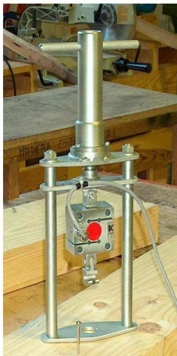
Fig. 3. Screw withdrawal force meter (Fakopp, Hungary)
