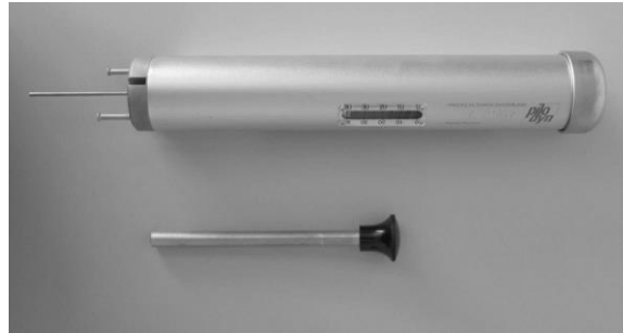
Fig. 2. Pilodyn 6J Forest device (Proceq, Switzerland)
