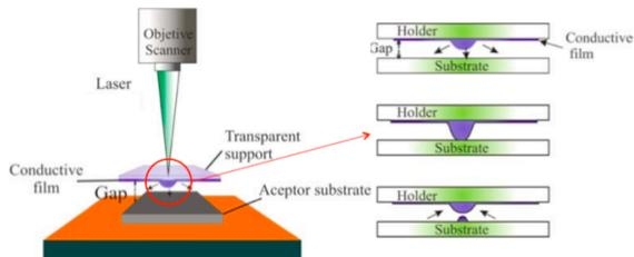
**Figure 1:** Principle of LIFT process for metallization of thin-film solar cells.
