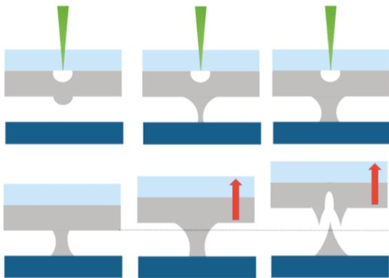
**Figure 2:** Scheme of the LIFT process for high viscosity pastes, showing the formation of paste column between donor and acceptor substrate, the donor removal and the final shape definition.
