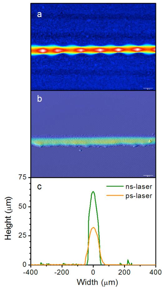
**Figure 3:** False-color confocal images of silver lines printed using (a) the ns- and (b) the ps-laser. (c) Transversal profiles of the lines shown above.
