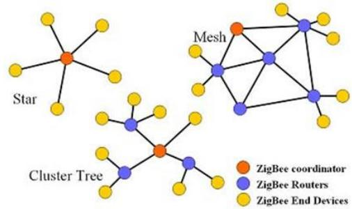
Fig. 2 Zigbee™ topologies
