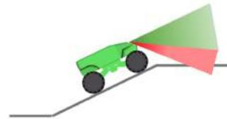
Fig. 6: Critical situation when the robot is over the bridge. The green beam shows the field of view of the on-board camera, which does not give a ground reference.
