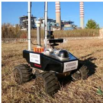
Fig. 5: Summit XL Robotic platform, including the equipment used in the challenge.
