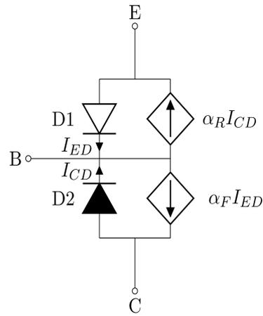
**Figure 2** Ebers-Moll model for the solar cell in dark conditions. Notice  $I_{ED}$  is the total current through the diode that forms the base-emitter junction and  $I_{CD}$  is the total current through the diode that forms the base-collector junction.  $\alpha_F$  and  $\alpha_R$  are the common-base current gains for the transistor operating in active-forward and active-reverse respectively.
