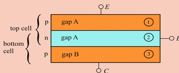
Simplified layer structure of the three terminal heterojunction bipolar transistor solar cell (3T-HBTSC).
