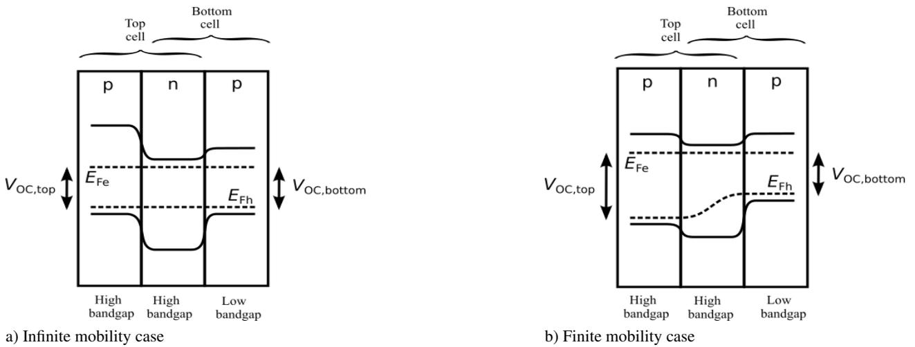
**Figure 3** Qualitative plot of the shape of the quasi-Fermi levels when the top and bottom cell are illuminated and in open-circuit and when a) infinite mobility is assumed and b) finite mobility for the holes is assumed.  $V_{OC,top}$  and  $V_{OC,bottom}$  indicate the open-circuit voltage of top and bottom cell respectively.
