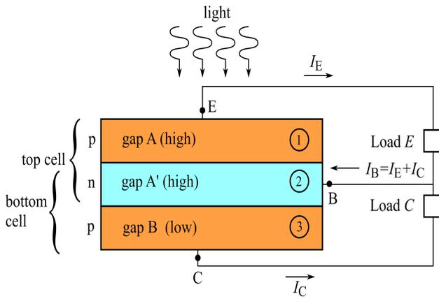
**Figure 1** Structure of a three terminal heterojunction bipolar transistor solar cell.
