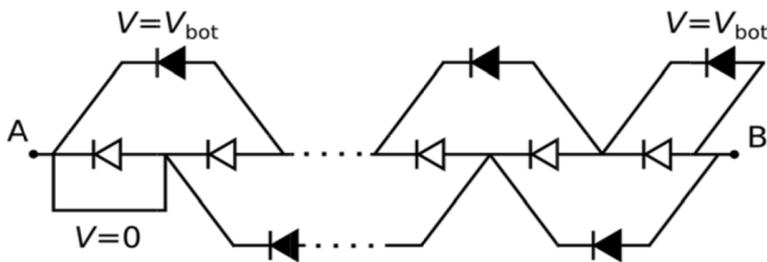
**Figure 5** Layout showing a possible cell interconnection at module level. The filled diodes represent the bottom cell. The hollow diodes represent the top cell.  $V_{bot}$  indicates the voltage of the bottom cell.  $A$  and  $B$  represent the two terminals of the module (Adapted from Gee [11]).
