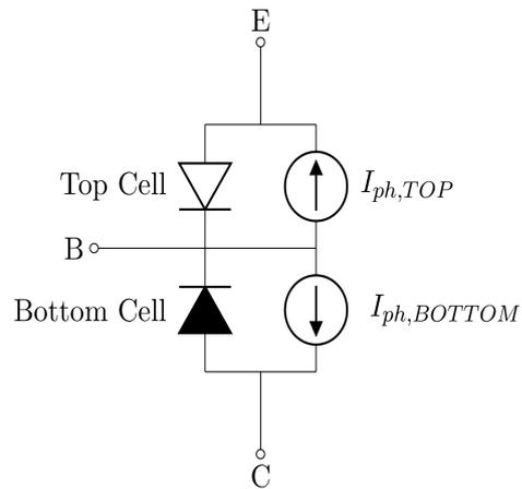
**Figure 4** Circuit model for the solar cell when transistor effects are removed.  $I_{EL}$  and  $I_{CL}$  are now photo-generated currents whose value depends on the illumination conditions.
