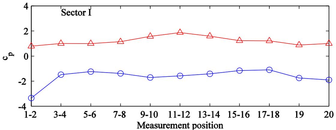
Figure 14 – Envelope of extreme wind loads on sector I
