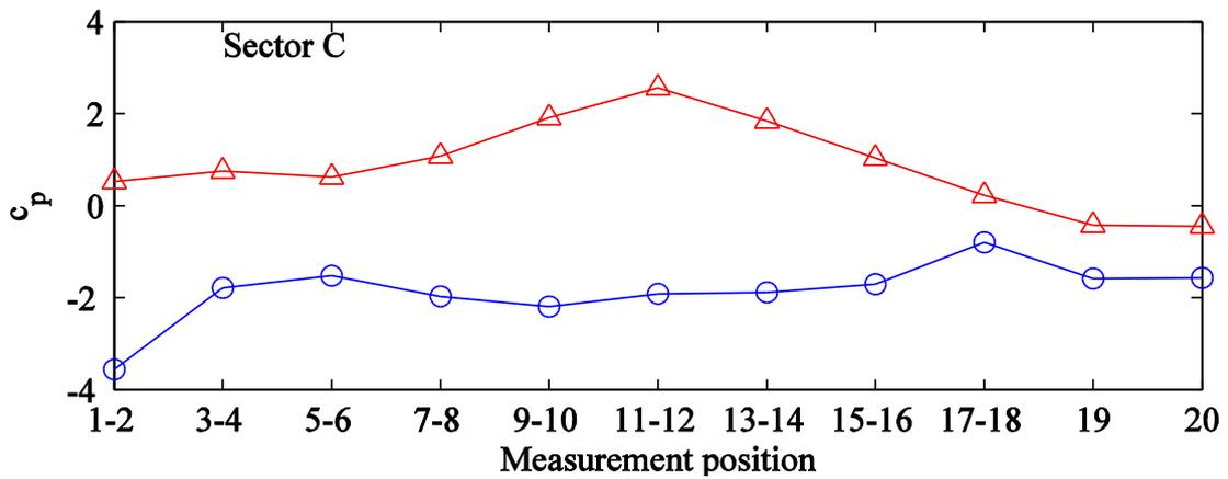
Figure 8 – Envelope of extreme wind loads on sector C
