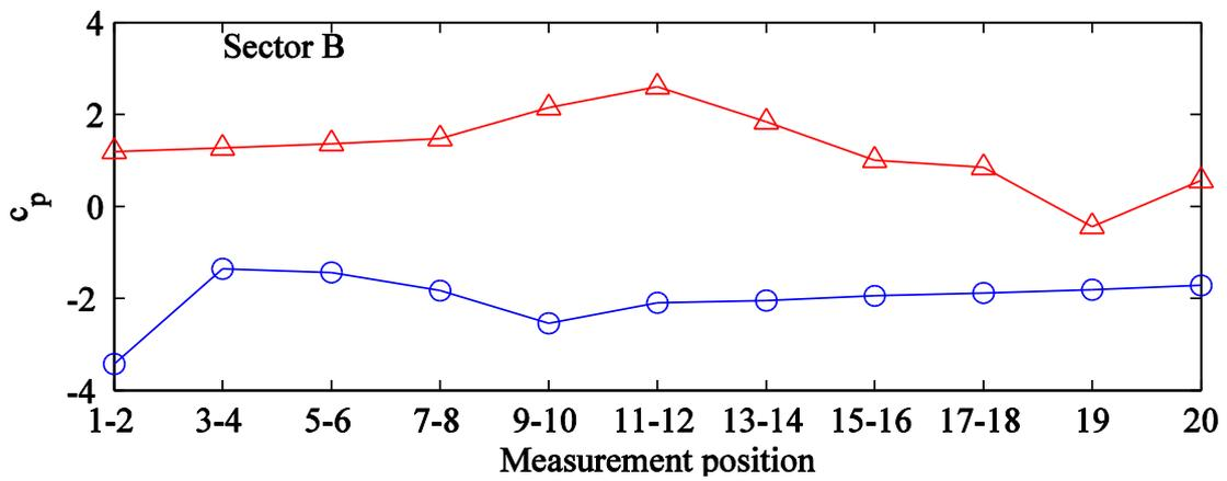
Figure 7 – Envelope of extreme wind loads on sector B
