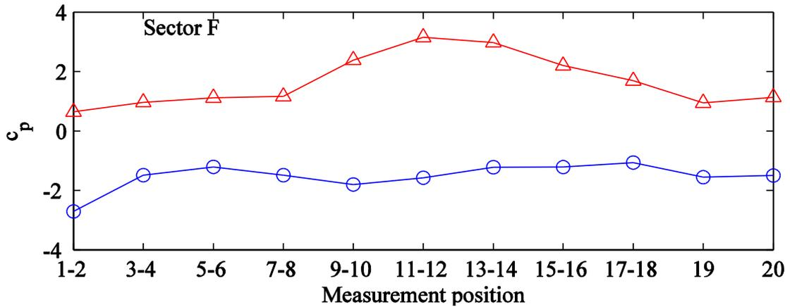
Figure 11 – Envelope of extreme wind loads on sector F
