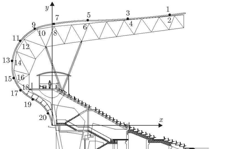
**Figure 2** – Position of the pressure taps on a segment. Taps 1-18 are placed in pairs (odd taps in the extrados, even taps in the intrados), and taps 19 and 20 are placed without their counterpart in the intrados
