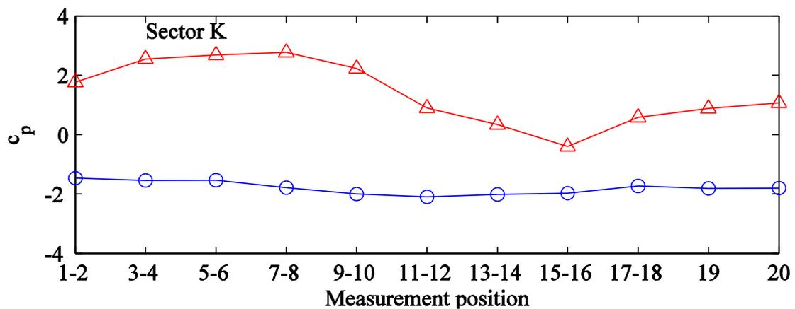
Figure 16 – Envelope of extreme wind loads on sector K
