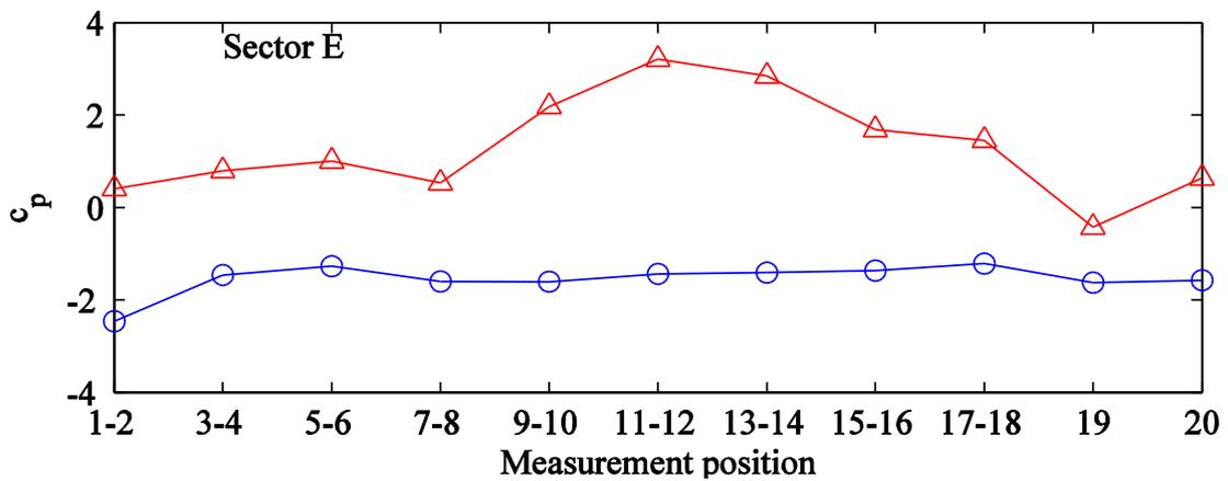
Figure 10 – Envelope of extreme wind loads on sector E
