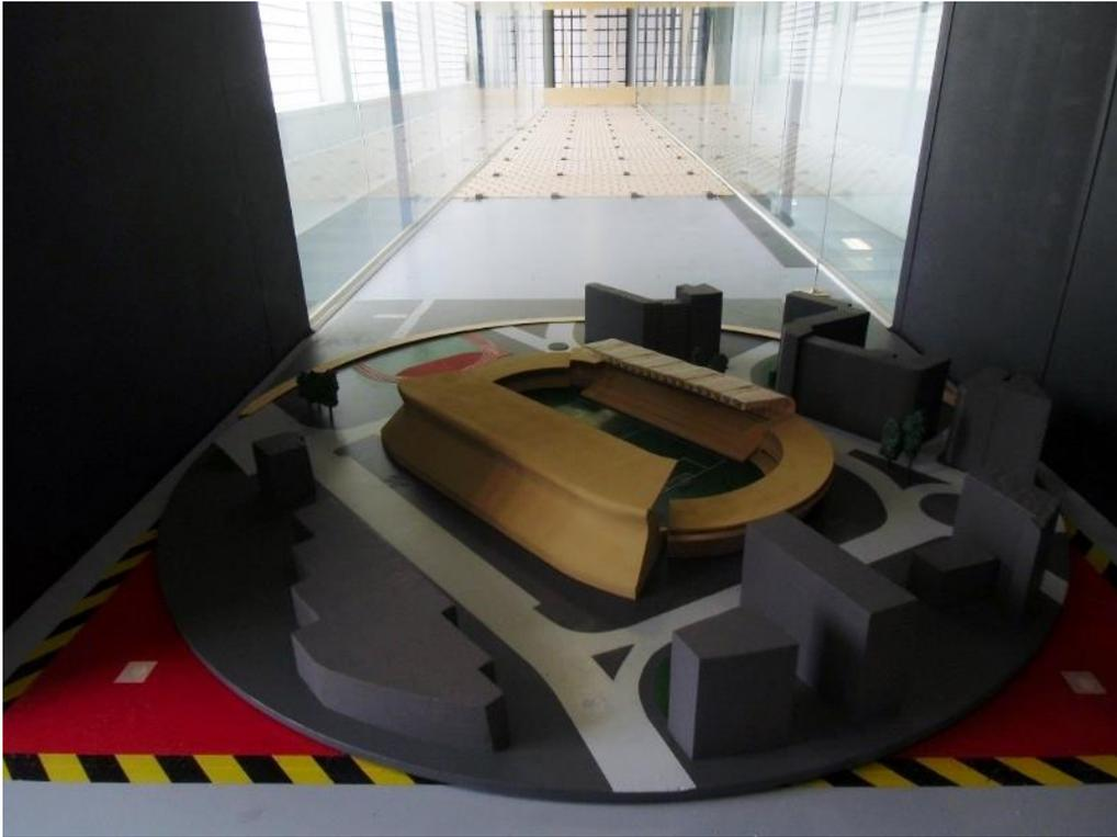
**Figure 1** – Picture of the model placed in the wind tunnel. Upstream, roughness elements reproducing atmospheric boundary layer can be seen
