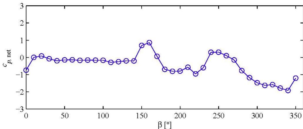
**Figure 5** – Net pressure coefficient for pair of taps 9-10 of segment A against the yaw angle of the wind
