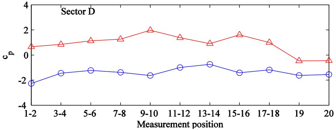
Figure 9 – Envelope of extreme wind loads on sector D
