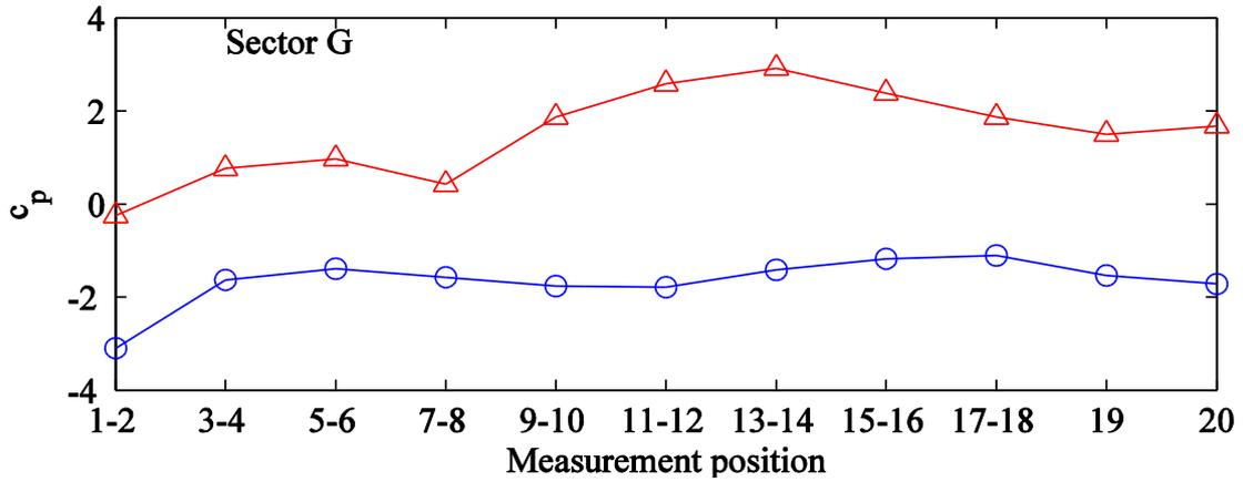
Figure 12 – Envelope of extreme wind loads on sector G
