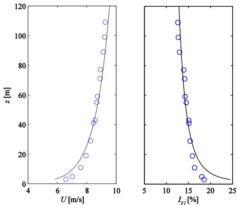
**Figure 4** – Vertical profile of wind velocity (left) and turbulence intensity (right) in the wind tunnel (blue circles) and in the Eurocode model (black line)
