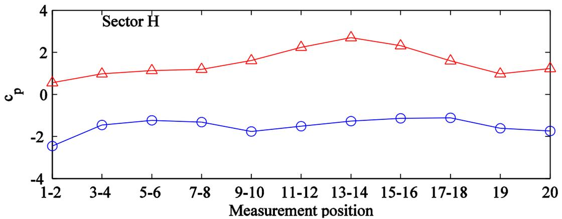
Figure 13 – Envelope of extreme wind loads on sector H
