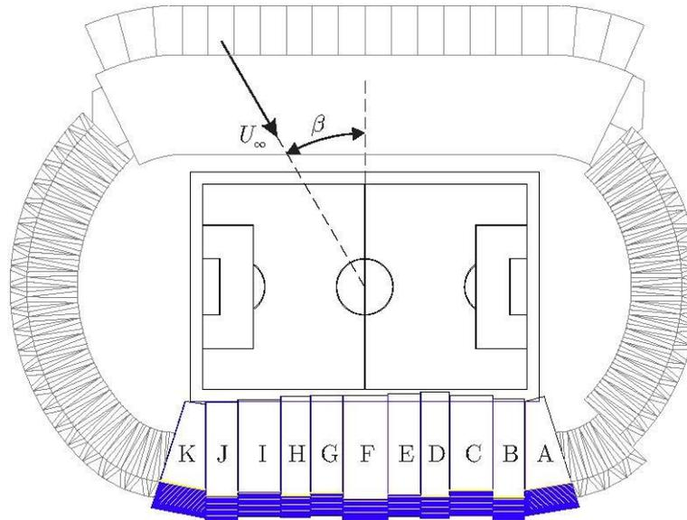
**Figure 3** – Naming of the eleven segments and definition of the yaw angle,  $\beta$
