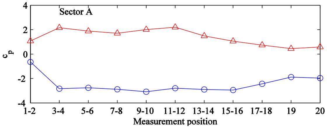
Figure 6 – Envelope of extreme wind loads on sector A
