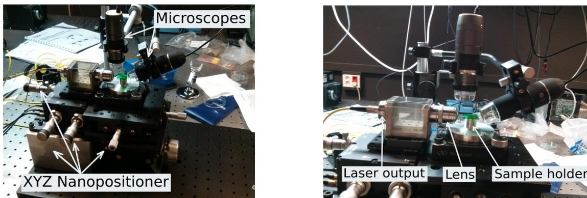
Figure 1. Different views of the X-Y-Z nanopositioner setup for coupling light to PICs.
