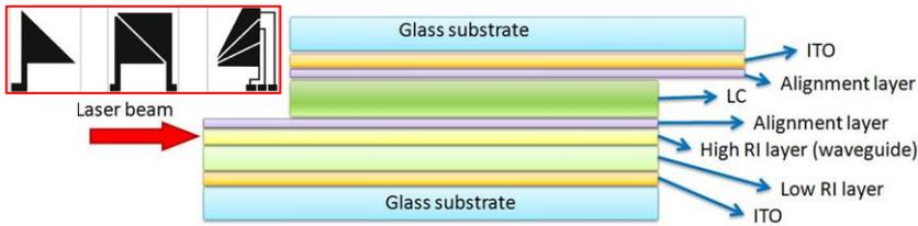
Fig. 1.- Planar beam steering cell. Inset, electrode design
