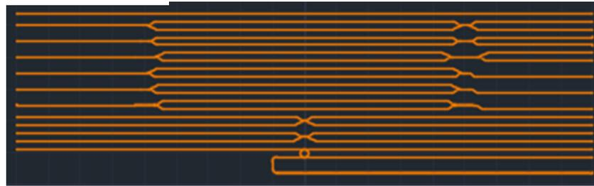
Fig. 2.- Several  $1.5 \times 0.5 \mu\text{m}$  waveguide structures for PICs.
