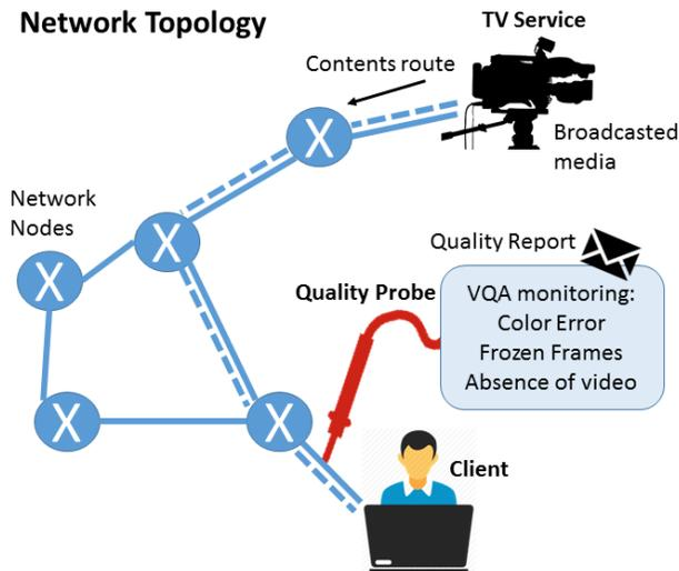
FIGURE 1. QUALITY PROBE IN NETWORK ARCHITECTURE
