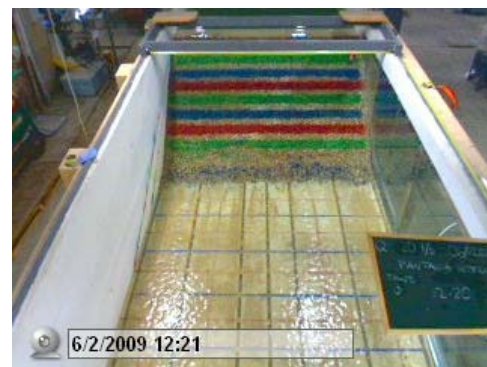
b) Visual measurement of the advance degree of failure with the help of coloured lines
