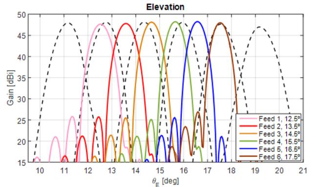
Fig. 6. Simulated radiation patterns for the bifocal antenna (solid lines) and the single-focus reference antenna (dashed lines).
