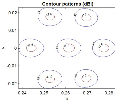
Fig. 7. Radiation pattern contours of 47.5 dBi and 45 dBi for the design beam and a ring of five beams.
