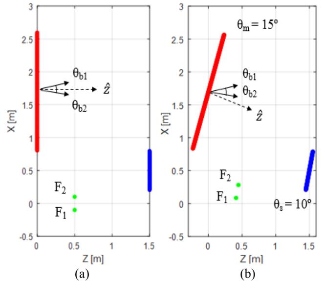
Fig. 3. Geometry of the dual reflectarray antenna: (a) with parallel reflectarrays, (b) after tilting both reflectarrays.
