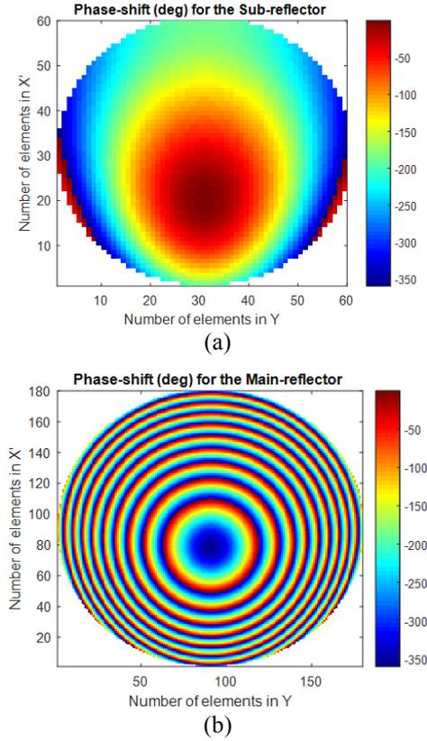
Fig. 4. Adjusted phase-shift distributions for (a) the sub-reflector and (b) the main reflectarray.
