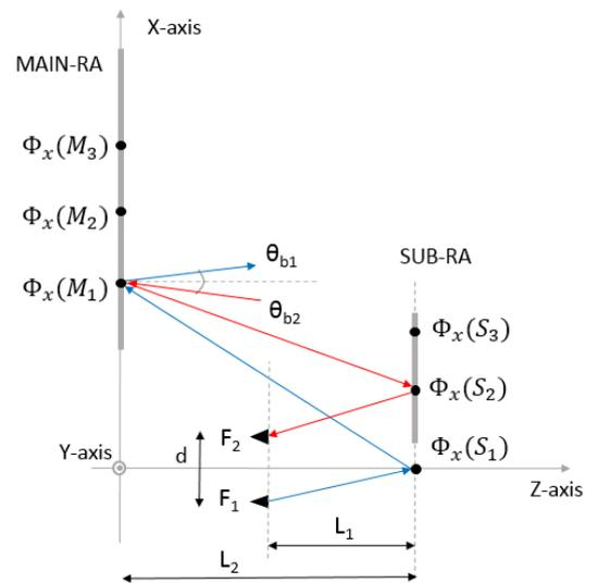
Fig. 1. Geometry and parameters of the bifocal dual reflectarray antenna.
