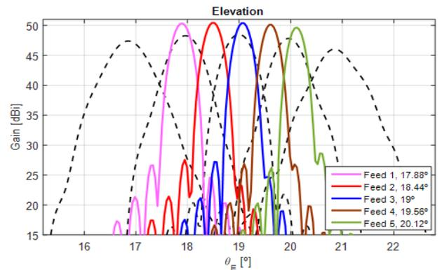
Fig. 8. Simulated radiation patterns for the bifocal antenna with  $0.56^\circ$  beam separation (solid lines) and the single-focus reference antenna (dashed lines).
