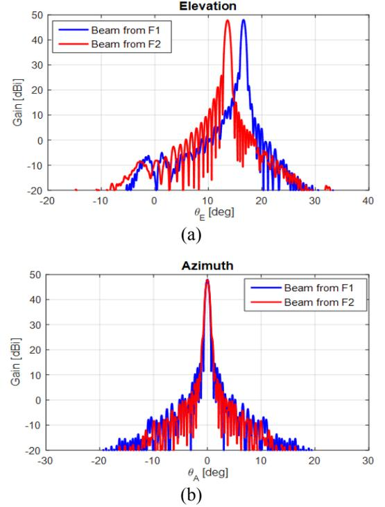
Fig. 5. Simulated radiation patterns for the dual reflectarray antenna after tilting both reflectarrays: (a) in elevation, (b) in azimuth.
