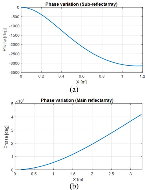
Fig. 2. Phase curves obtained by the bifocal technique for (a) the sub-reflectarray and (b) the main reflectarray.
