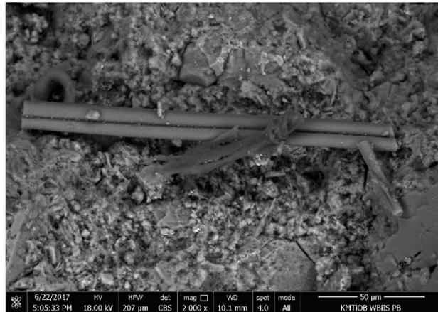
**Fig. 2: SEM micrographs of a cement mortar with the incorporation of 30% mixed waste of mineral wools.**
