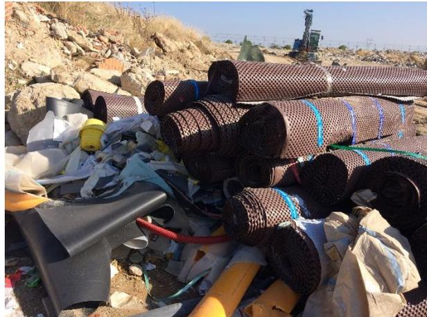
**Fig. 1:** Residues of mineral wool stored in the Complex Treatment of Construction and Demolition Waste located in El Molar.
