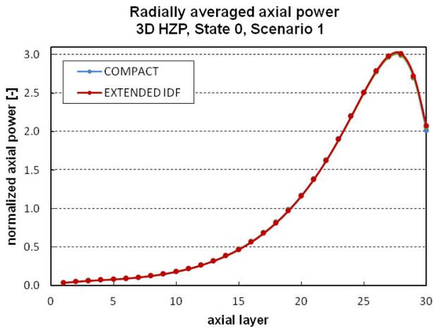
Fig. 9. Axial power distribution at HZP for VVER
