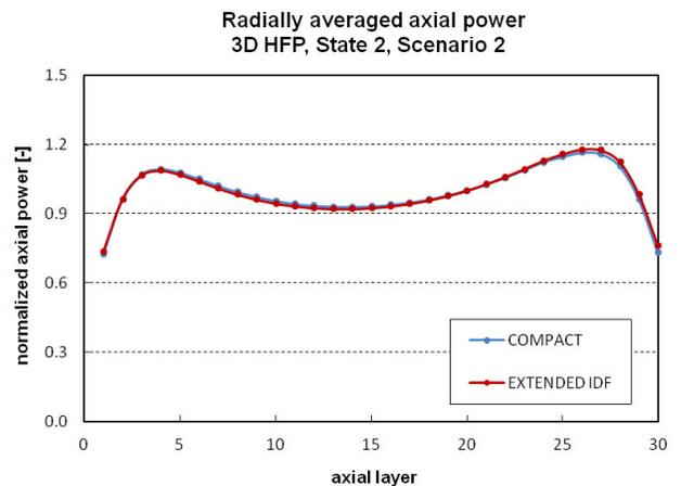
Fig. 10 Axial power distribution at HFP for VVER
