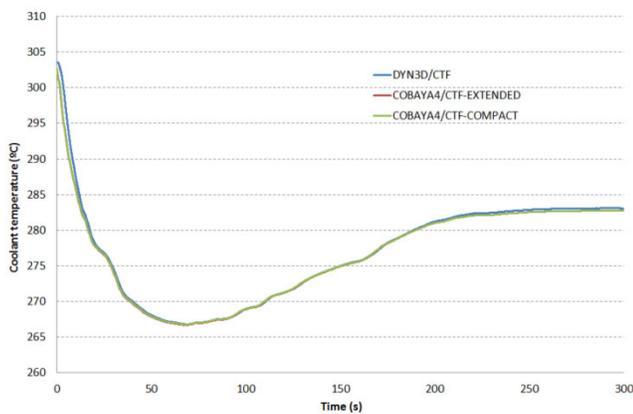
Fig. 16. Core average coolant temperature evolution during the MSLB transient in a VVER
