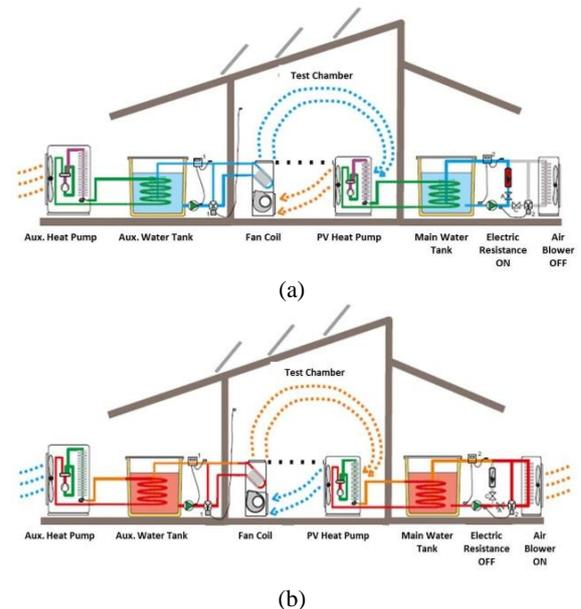
**Figure 2:** Schematic of the PV heat pump installation tested, operating in cooling (a) and heating (b) modes.
