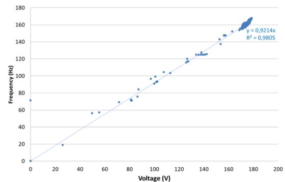
**Figure 4:** Output frequency versus voltage for one of the phases of the frequency converter.
