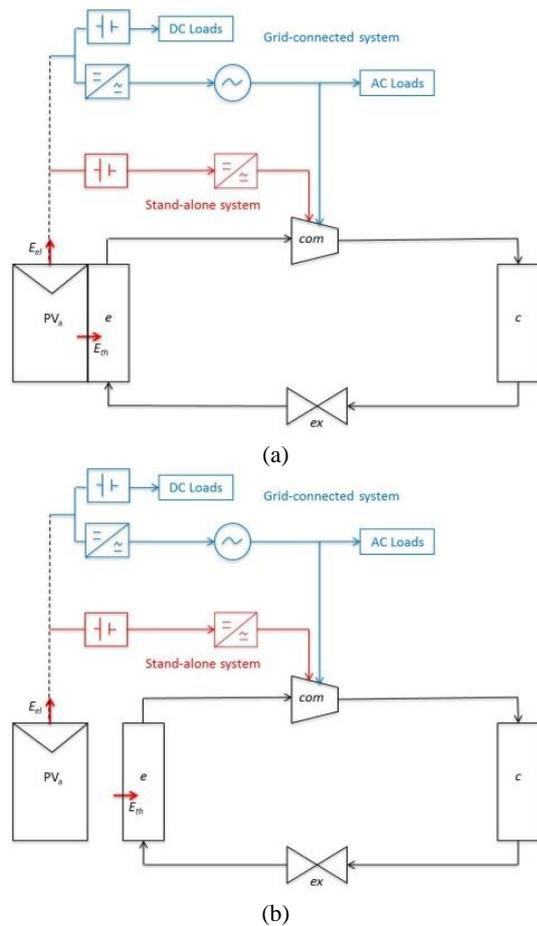
**Figure 1:** Schematic of a basic PVT (a) and OPV (b) heat pump system with grid-connected and stand-alone configurations.
