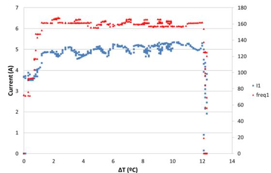
**Figure 5:** Output frequency and electric current versus  $\Delta T$  for one of the phases of the frequency converter.
