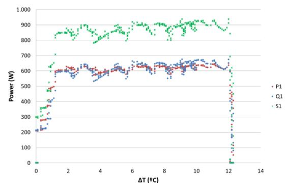
**Figure 6:** Active, reactive and total power versus  $\Delta T$  for one of the phases of the frequency converter.
