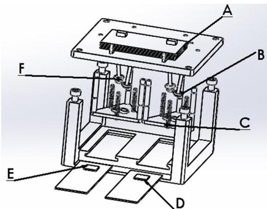
Figure 2. A-Electronic unit; B- Optical Signal channel; C- Optical Alignment mount; D- Signal FPI; E- Reference FPI; F- Optical Reference channel.
