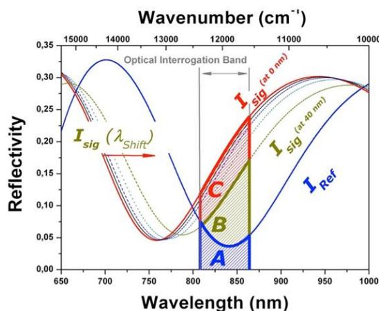
Figure 1. IROP-based read-out system theoretical behavior
