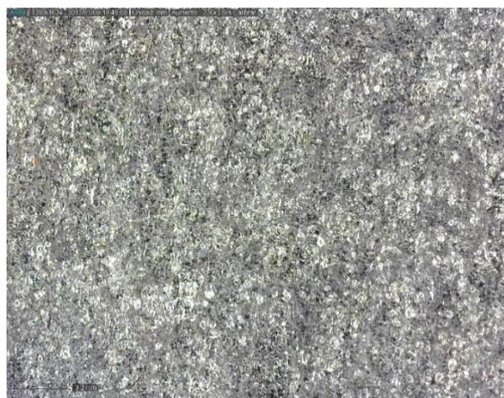
Fig. 2. Al 6061 microscope image (x220) after 40 days in anodic solution at 70 °C.
