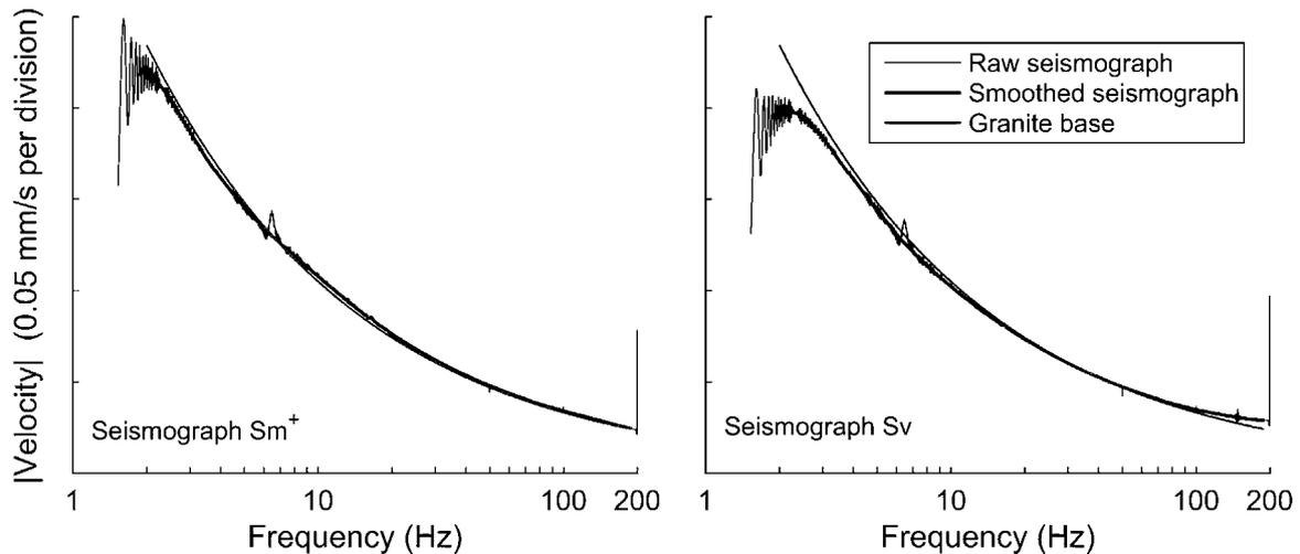
Fig. 2. Amplitude spectra of both seismographs for trial No. 2 in test series GG20.
