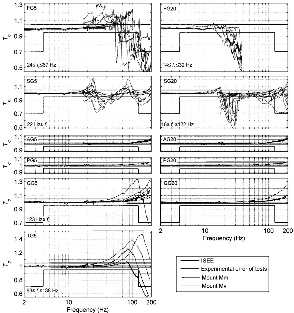
**Fig. 4.** Coupling transmissibility for free (FG5, FG20), sandbagged (SG5, SG20), anchored (AG5, AG20), plastered (PG5, PG20), glued (GG5, GG20), and taped (TG5) mounts on granite (the first letter of the test code is the coupling method – F: free; S: sandbagged; A: anchored; P: Plastered; G: Glued; T: Taped–, the second one is the base –G: granite–, and the number is the peak velocity);  $f_r$  is the frequency of the first peak or resonance frequency.
