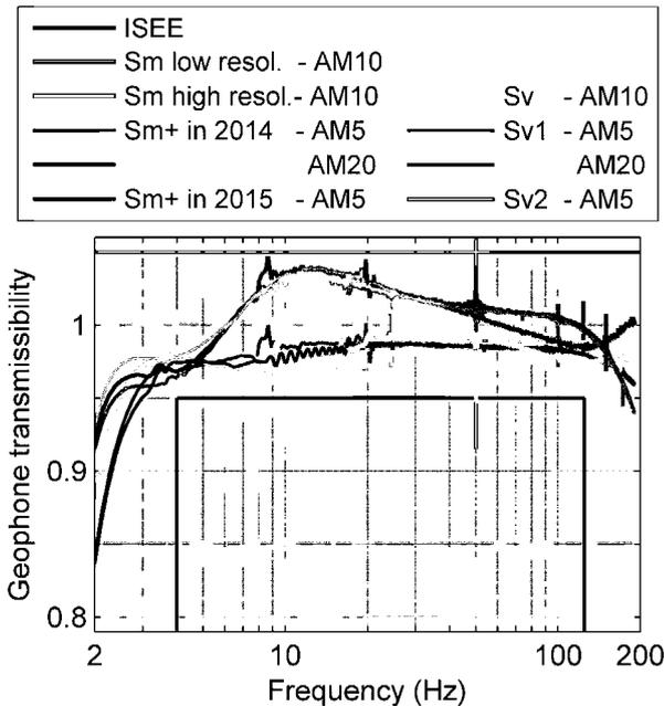
Fig. 3. Mount-to-geophone transmissibility of the seismographs tested; AM10 was made in the first campaign, and tests in 2014 and 2015 correspond to the second and third campaign, respectively.
