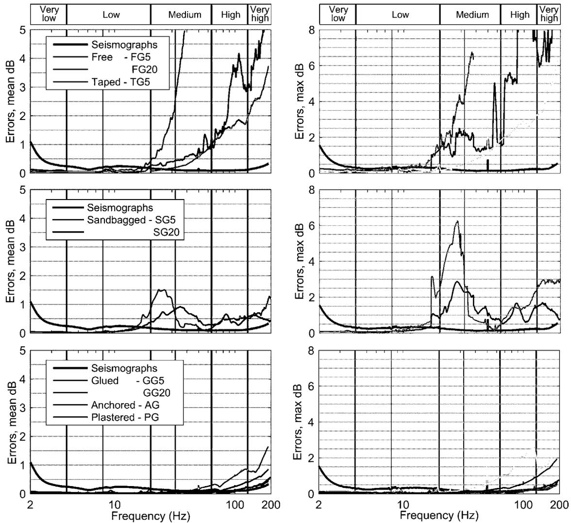
**Fig. 5.** Errors: expected (left graphs) and maximum (right graphs) for each test series (the first letter of the code is the coupling method – F: free; S: sandbagged; A: anchored; P: Plastered; G: Glued; T: Taped–, and the second one is the base –G: granite). Vertical scales are different for left and right graphs; vertical thick lines show the bounds of the frequency intervals considered, being from left to right 4, 8, 20, 32, 64 and 128 Hz.
