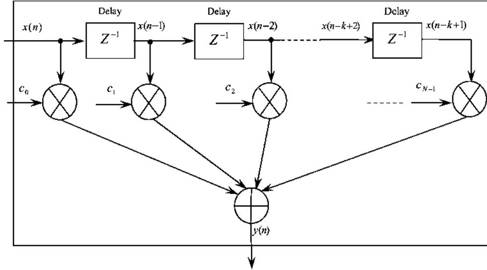
Fig. 2. An  $N$ -tap digital FIR filter.
