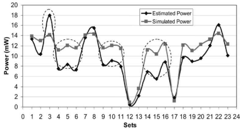
Fig. 4. Power comparison between macro-model and reference simulated power. Larger error spots for metric values between [0, 0.2] or [0.8, 1].
