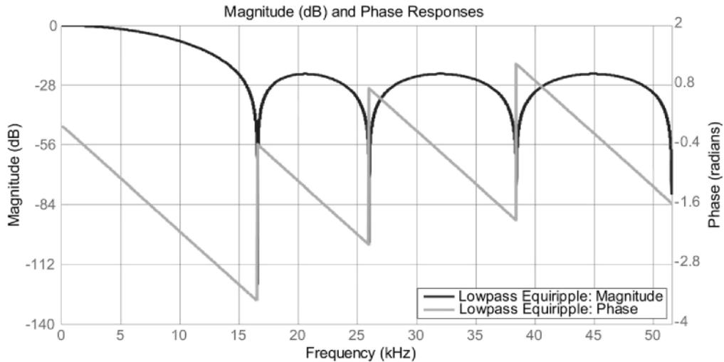
**Fig. 3.** Magnitude and the phase response of the FIR filter.
