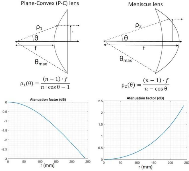
Fig. 3 Geometry of the plane-convex and meniscus lens and their corresponding amplitude correction factors
