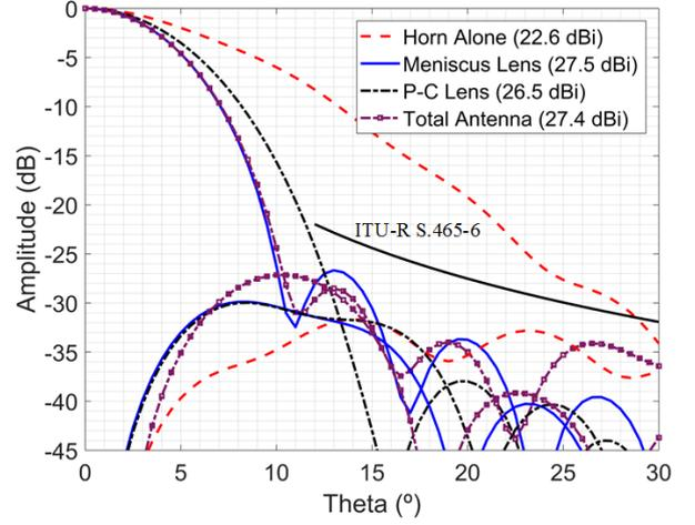
Fig. 5. Phi=45° cut radiation pattern for the horn with and without lens, and for the complete antenna
