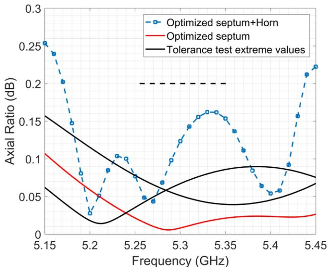
Fig. 2 Axial Ratios of the optimized septum, worst cases of the tolerance test and complete antenna
