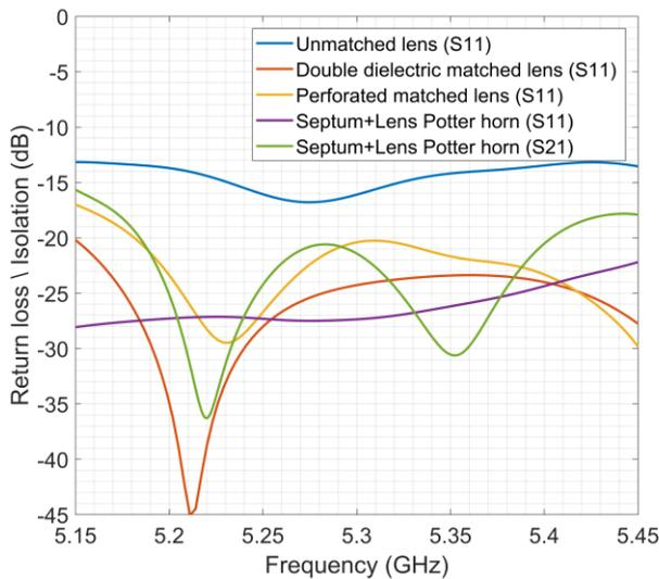
Fig. 7 Return loss and isolation for several meniscus lens matching configurations and for the complete antenna
