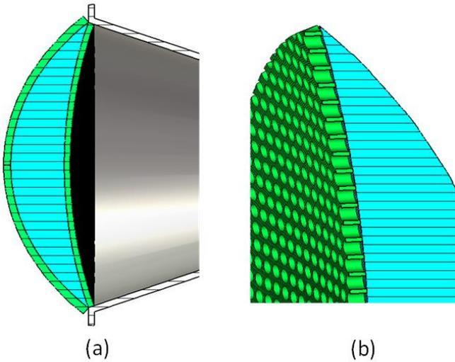
Fig. 6 Sectional views of a horn: (a) with two dielectric adaptation layers and (b) final optimized lens
