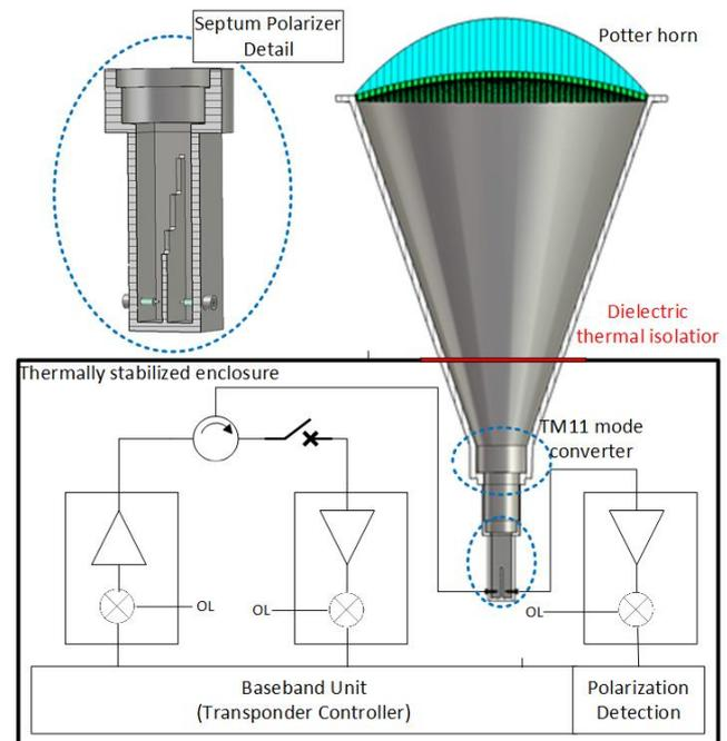
Fig. 1 Block diagram of the ASCAT radar echo calibrator
