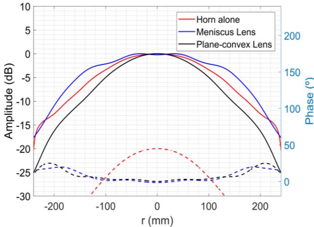
Fig. 4 Aperture field amplitude (continuous trace) and phase (dotted) of the horn with and without lens
