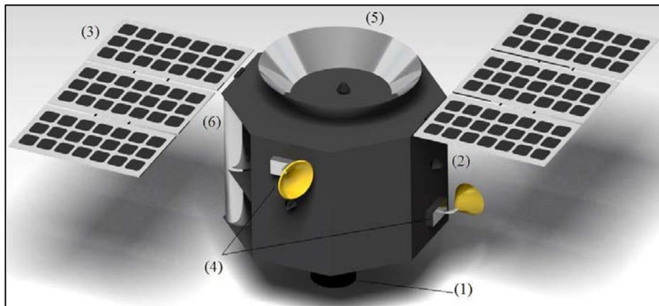
Finally, for earth communication, a double system was selected: a S-band antennae system (with 5 S-band antennae distributed around the spacecraft structure) for GTO orbit and WBS transfer; and a 2 X-band steerable antennae system for Moon orbit. The main ground station and mission control will be located in Madrid, Spain (40.42°N, 3.79°W) although some other ground station options could be required to support the mission.
