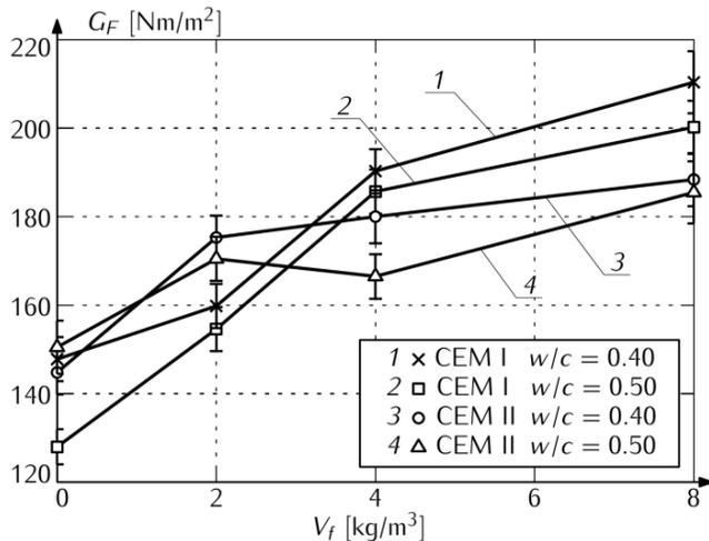
Fig. 7. Effect of fiber volume fraction  $V_f$ (%), cement type and  $w/c$  ratio on fracture energy  $G_F$ .
