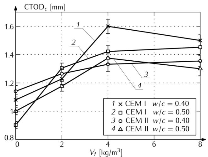
Fig. 6. Effect of fiber volume fraction  $V_f$  (%), cement type and  $w/c$  ratio on  $CTOD_c$ .
