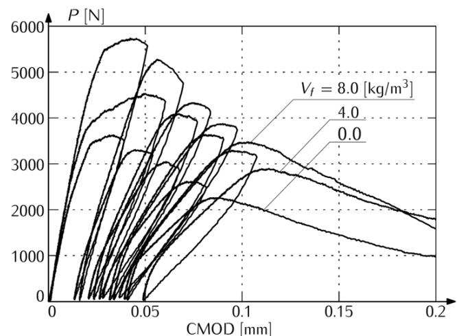
Fig. 3. Load  $P$ - $\text{CMOD}$  plots for concretes with  $w/c = 0,40$  (CEM I 42,5 R) with different content of basalt fibers  $V_f$ .
