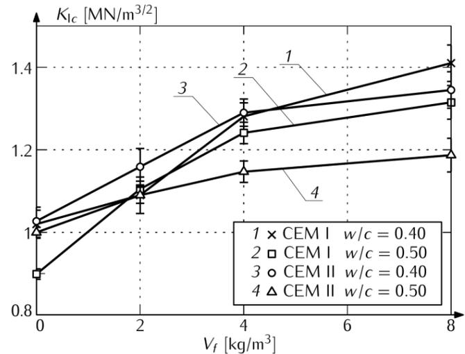
Fig. 5. Effect of fiber volume fraction  $V_f$  (%), cement type and  $w/c$  ratio on fracture toughness  $K_{Ic}$ .
