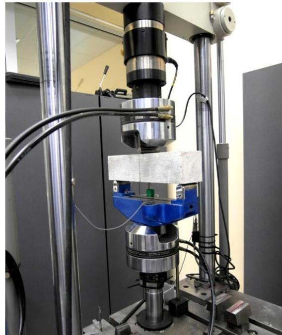
Fig. 2. Notched beam specimen during testing.
