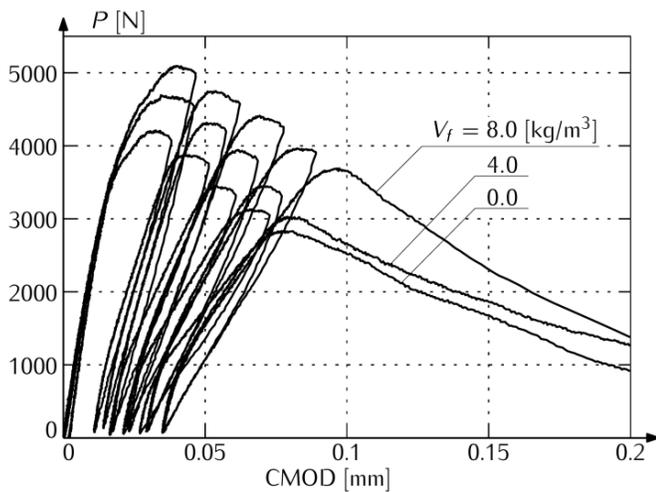
Fig. 4. Load  $P$ -CMOD plots for concretes with  $w/c = 0,40$  (CEM II/A-V 42,5 R) with different content of basalt fibers  $V_f$ .
