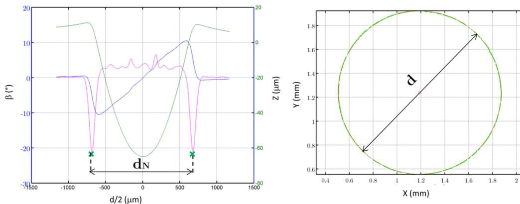
Fig. 3. Brinell diameter determination for an indentation profile  $N$  (left) and for a complete circumference of the edge (right).
