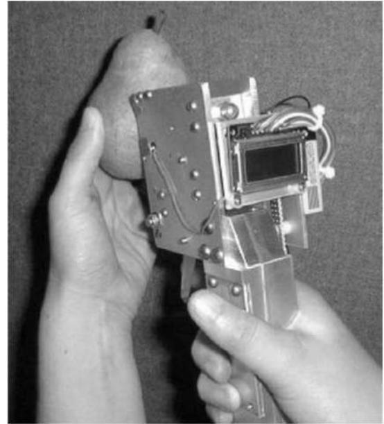
Figure 2. First prototype of the handheld impact firmness sensor (Chen and Thompson, 2000).
