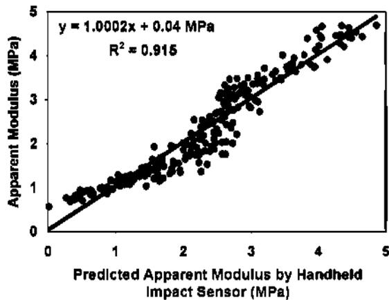
Figure 4. Validation results for the handheld impact firmness model using  $(1/t)^{2.5}$  and  $(A/t)^{1.25}$  terms to predict whole-pear apparent modulus.
