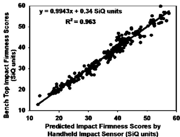
Figure 5. Validation results for the handheld impact firmness model using  $1/t$  and  $A/t$  terms to predict whole pear firmness as determined by a commercial benchtop impact firmness instrument.
