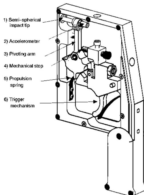
Figure 3. Illustration of the improved prototype showing the redesigned, mechanically counterbalanced impact arm (signal conditioning circuitry, microprocessor, and display not shown for clarity).
