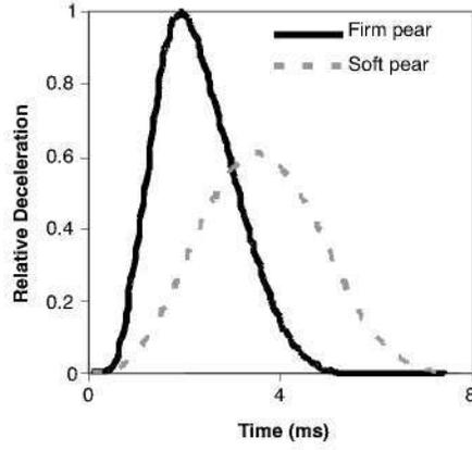
Figure 1. Impact response curves of a low-mass rigid semi-spherical impact arm tip from the handheld sensor on soft and firm 'Bartlett' pears.
