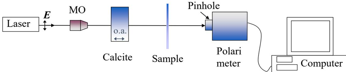
Fig 1. Experimental setup
