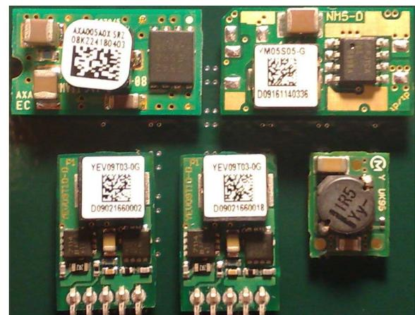
Fig. 10. Actual power architecture built with VR block modules
