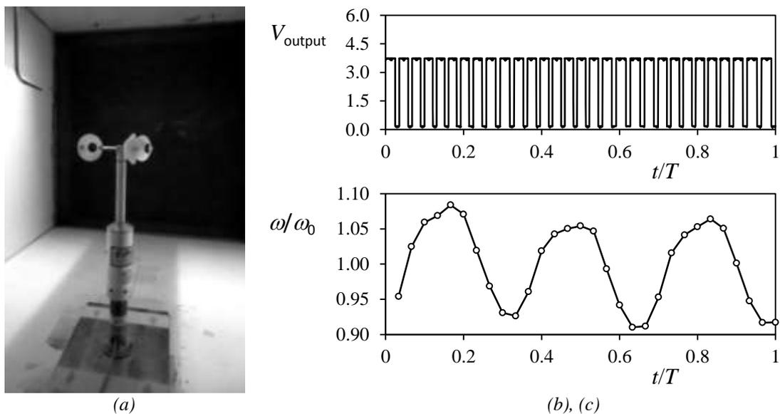
Figure 2. (a) Cup anemometer being calibrated at the IDR/UPM Institute wind tunnel, (b) Train of pulses (voltage signal,  $V_{\text{output}}$ ) along one turn, (c) Variations of the rotor speed rate in relation to the average rotation rate,  $\omega/\omega_0$ , along one turn. From [61].
