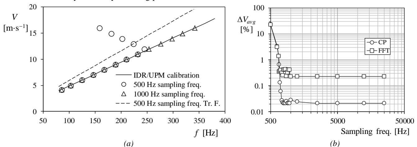
Figure 3. (a) Points (output frequencies) calculated with 500 and 1000 Hz sampling frequency 25-second large datasets. The transfer function based on the points calculated with 500 Hz sampling frequency dataset and the proper calibration of the cup anemometer are also included, (b) Averaged value of the transfer function error of calibrations performed by calculating the anemometer output frequency using CT and FFT.
