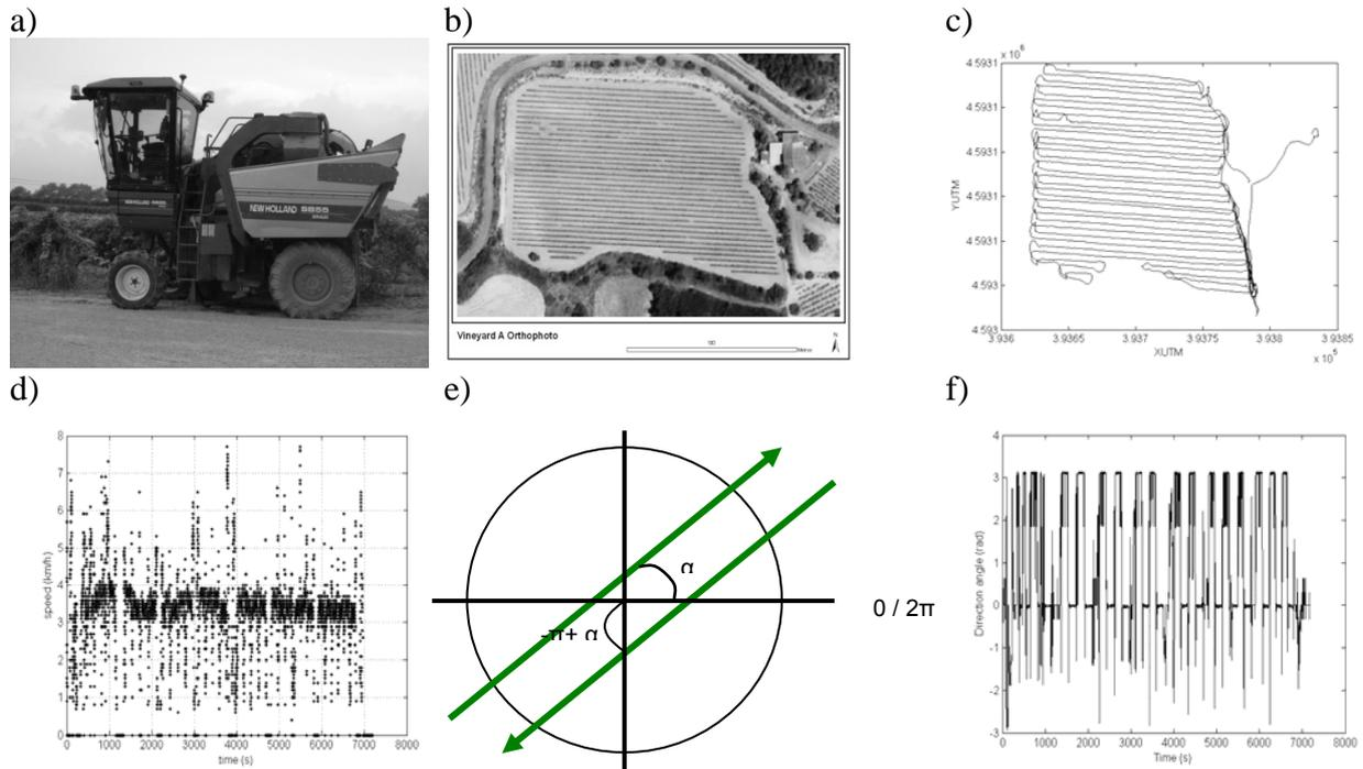
Figure 1: a) Photograph of the grape harvester New Holland SB55; b) Example of an orthomosaic; c) Example of XUTM and YUTM coordinates; d) Example of the grape harvester speed; e) and f) Identification of row crops.
