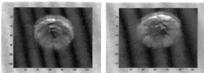
**Figure 6** MRI examples (type 1) of seedless oranges and oranges containing seeds at different belt speeds.
