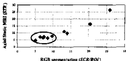
Figure 4 Comparison of automated MRI segmentation (nondestructive) under static conditions and RGB segmentation (destructive). Values of seedless oranges and oranges containing one seed are within the ellipse.
