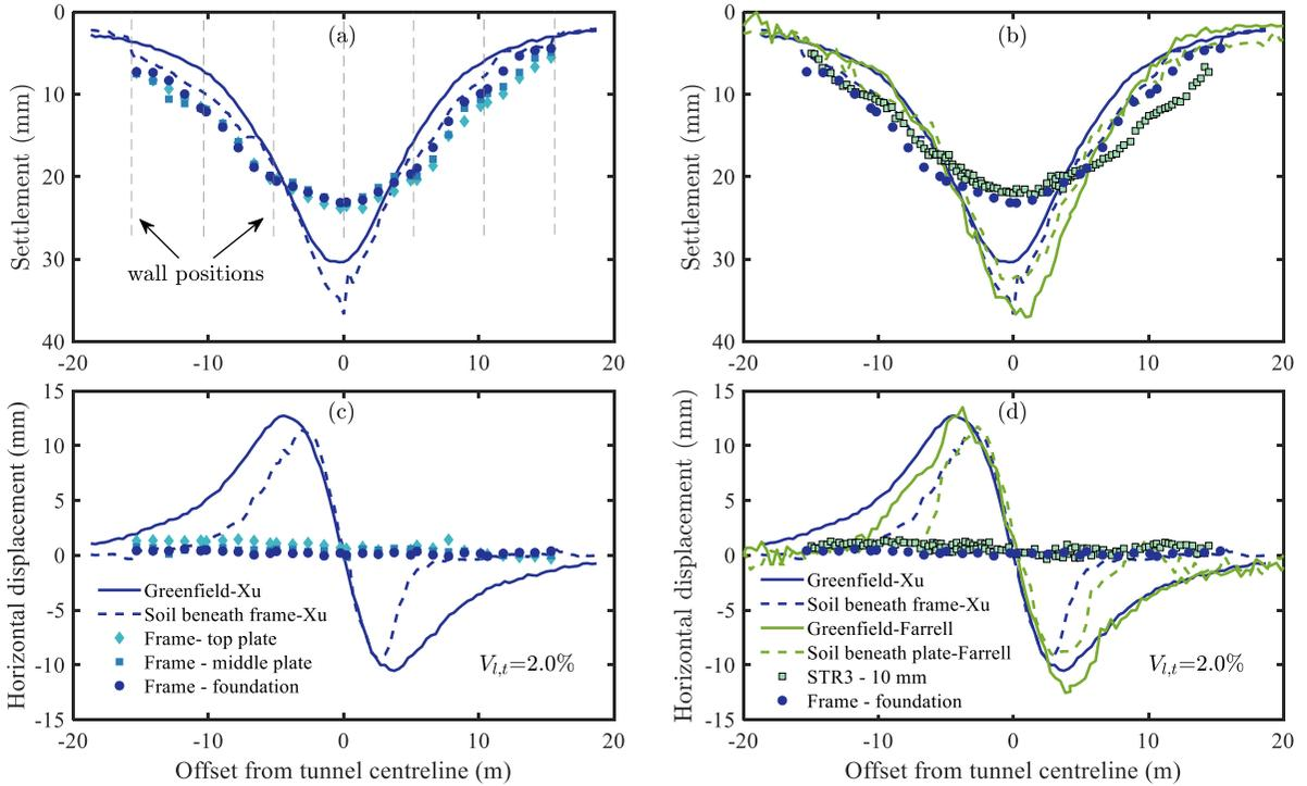
Figure 3 Experimental result and comparison with centrifuge data obtained by Farrell (2010).
