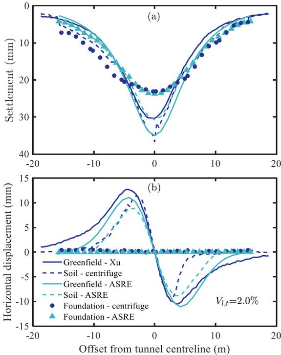
Figure 4 Experimental results and Class A predictions from the simplified numerical model.
