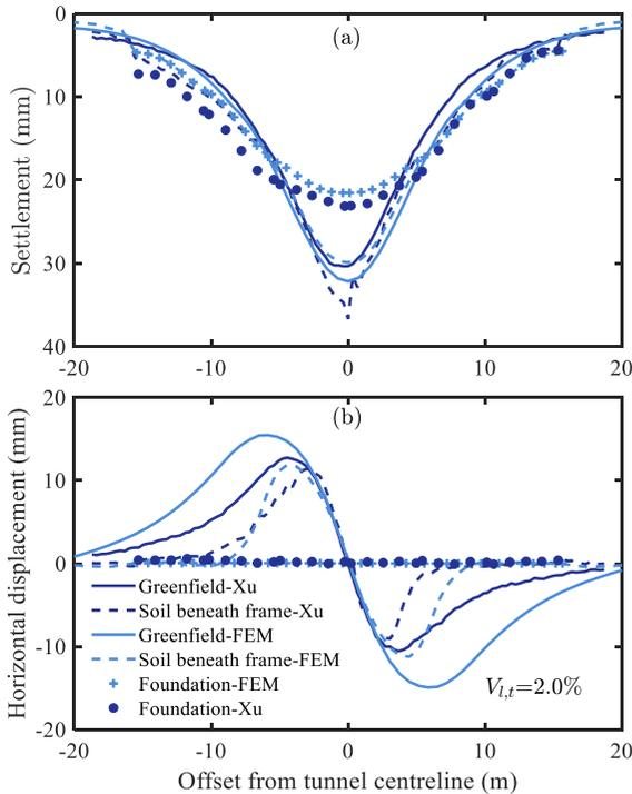
Figure 5 Experimental results and Class C predictions from the advanced numerical model
