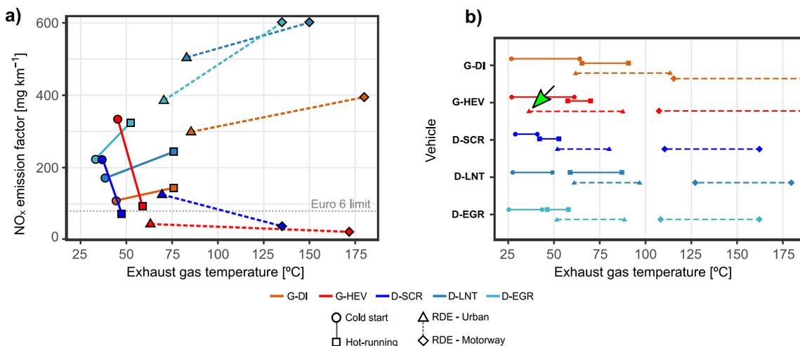
Figure 4. Exhaust gas temperatures for each vehicle and test, engine-off periods were not taken into consideration a) raw distance-specific emission factors and average exhaust gas temperature b) endpoints of horizontal lines represent 5th and 95th percentiles of test.
