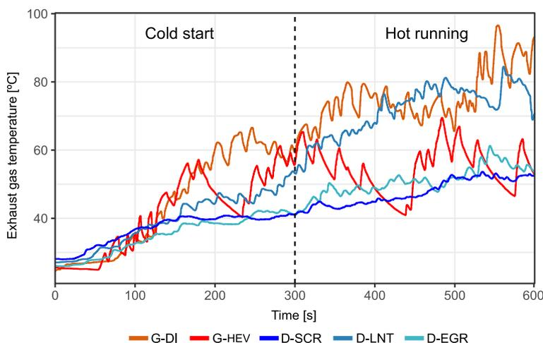
Figure 2. Exhaust gas temperature profiles during cold start (CS) and hot-running (HR) tests.
