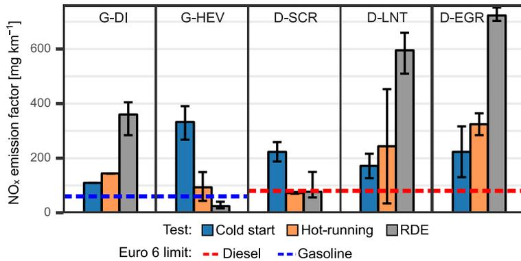
Figure 3. Average emission factors of cold start (CS), hot-running (HR) and RDE tests. Error segments represents maximum and minimum tests values.
