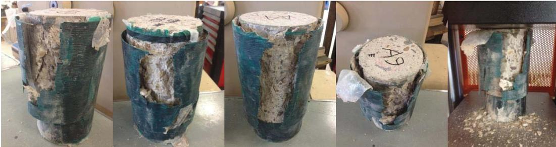
**Fig. 1:** *Break shape of confined concrete.*
