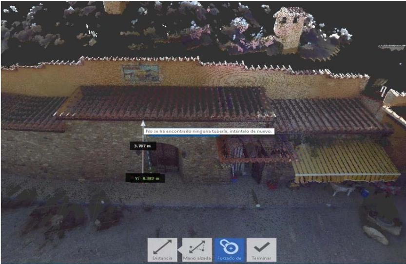
With the technique of three-dimensional digitalization, it can be obtained a 3D model of point cloud [2]. Later, with an appropriate educational software [3], we may get linear 3D models (models in BIM), necessary to simulate their behavior, such as quality of air (ventilation). Although mainly these are used to demonstrate that the necessary habitability requirements have been achieved in any type of housing and to compare them with the on-site data collection,
