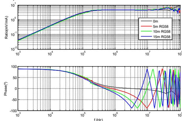
**Fig. 3: Transfer impedance versus cable length of its coaxial cable.**
