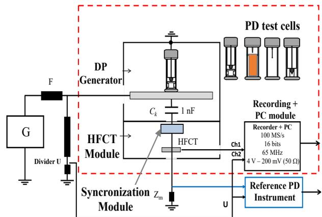
**Fig. 4: Configuration of the system for the characterization of measurement systems and PD diagnostics.**
