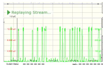
**Fig. 6: Measurement of charge and instants of the DP pulses measured with the reference system**
