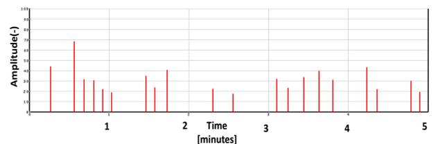
**Fig. 7: Train of reference PD pulses after removing electrical noise signals.**
