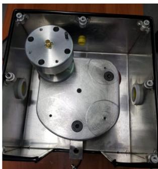
**Fig. 5: Module of the test cells for the generation of trains of PD pulses waveforms.**
