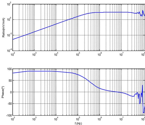
**Fig. 2: Measurement result of the transfer impedance of a commercial HFCT: Gain and angle shift.**
