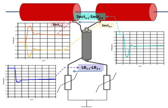
Fig. 4: Wave-shapes in per unity values, of measured voltages at sectionalizing joint and at SVL's terminals. Case of a Cross-Bonding configuration, with 10m of coaxial bonding lead and SVL1.
