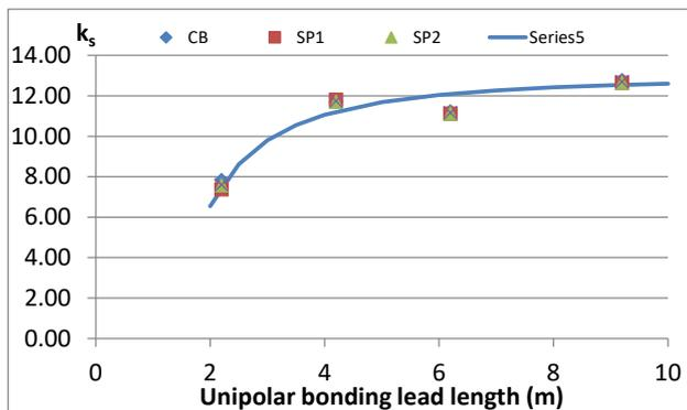
Fig. 4 Average value of  $k_s$  factor and fitting curve, obtained for all tests carried out with unipolar bonding lead (formulas (3) and (4)).
