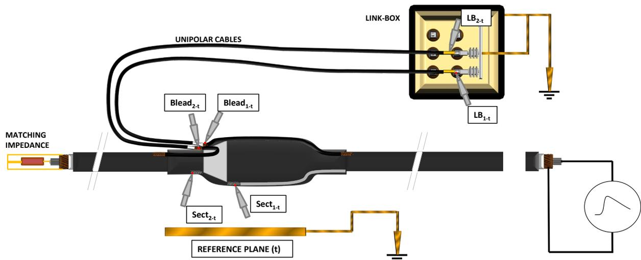
Fig. 1.b. Test setup for unipolar bonding lead.
