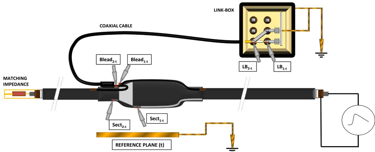
Fig. 1.a. Test setup for coaxial bonding lead.
