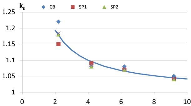
Fig. 3 Average value of  $k_s$  factor and fitting curve, obtained for all tests carried out with coaxial bonding lead (formulas (1) and (2)).
