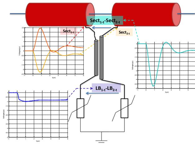
**Fig. 5: Wave-shapes in per unity values, of measured voltages at sectionalizing joint and at SVL's terminals. Case of a Cross-Bonding configuration, with 9.2m of unipolar bonding lead and SVL<sub>1</sub>.**
