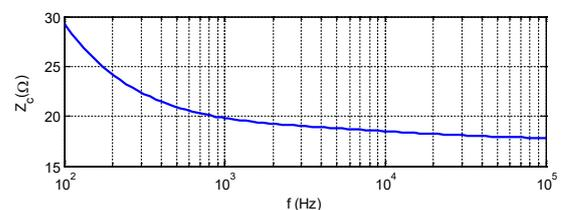
Fig. 2 Characteristic impedance  $Z_1$  of the power cable versus frequency.
