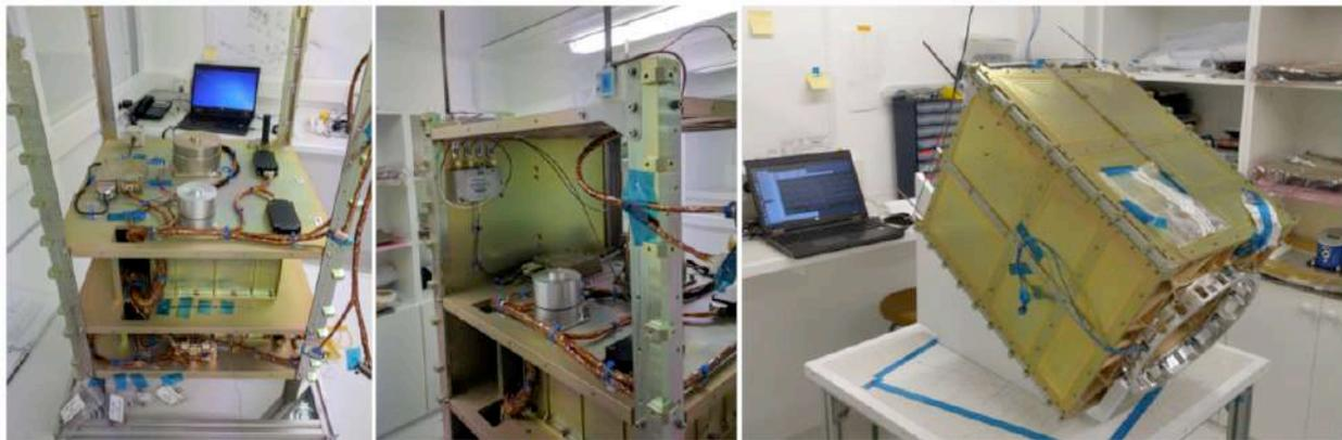
**Figure 11: Assembly and Integration campaign of the UPMSat-2. From left to right: integration of the payloads tray, integration of the upper tray of the satellite and verification of the ADCS subsystem at the end of the campaign.**
