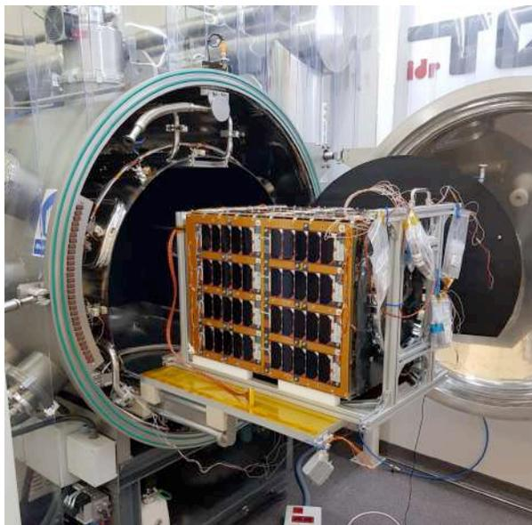
**Figure 14: The UPMSat-2 Flight Model during the thermal test campaign within IDR/UPM facilities.**
