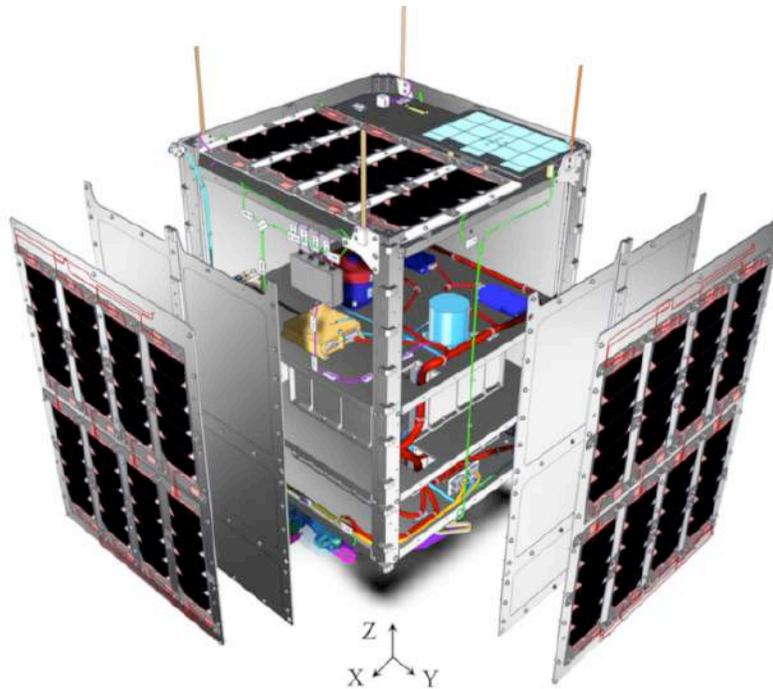
**Figure 1: UPMSat-2 microsatellite flight model CAD detail.**
