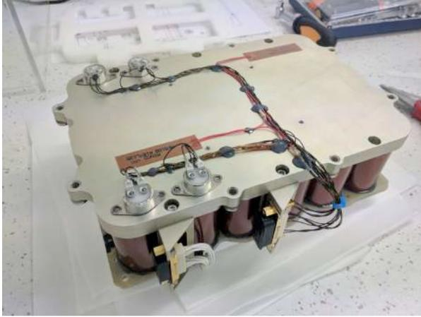
**Figure 7: Thermal control harness of the UPMSat-2 Li-Ion battery.**
