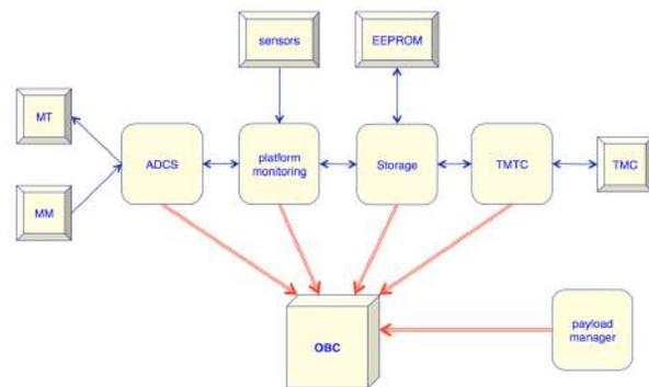
**Figure 9: UPMSat-2 software architecture**
