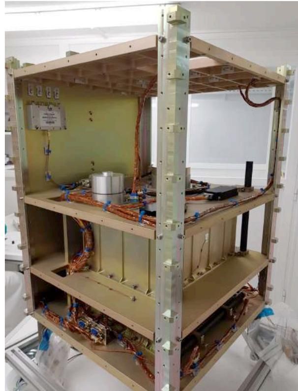
**Figure 4: Interior picture of the UPMSat-2 during the AIT campaign in the IDR/UPM ISO 8 clean room.**
