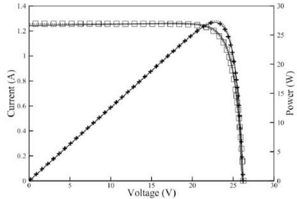
**Figure 6: Comparison between measurements and simulations of the  $I-V$  and  $P-V$  curves of a UPMSat-2 lateral panel. (---□---)  $I-V$  and (---+---)  $P-V$  curves measured during an illumination test of the solar panels; (—)  $I-V$  and (---)  $P-V$  curves simulated with a 1-diode/2-resistor model<sup>2</sup>**
