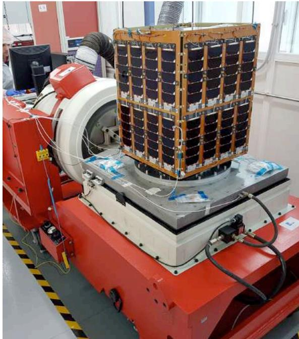
**Figure 12: UPMSat-2 during mechanical testing campaign in the IDR/UPM facilities.**
