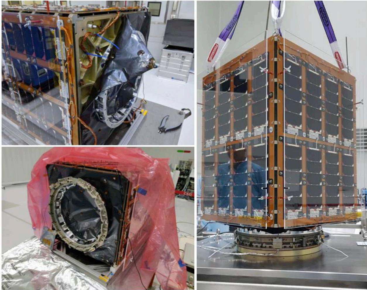
**Figure 16: Upper left picture, the finalization of the solar panels flight harness; bottom left, the installation of the upper ring of the separation band (MLB, Mark II Motorized Lightband, of Planetary System Corporations) and right picture, the UPMSat-2 MLB (upper and bottom rings) fully integrated.**
