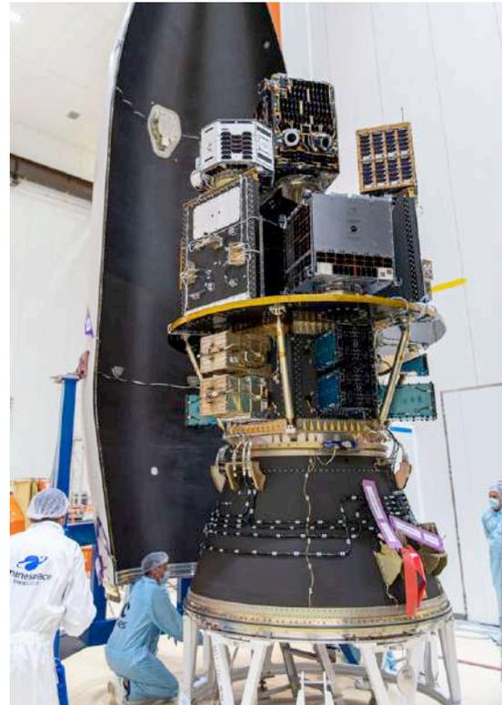
**Figure 15: Small Satellites Mission Service (SSMS) module integrated into the Payload Adapter, just before encapsulation of the Vega Fairing (Image Credit: Arianespace).**
