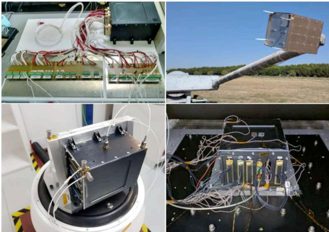
**Figure 10: Upper left picture, the EM model of the UPMSat-2; upper right, the STM model of the UPMSat-2 in the *ground-reflection antenna range* testing campaign; bottom left, the QM model of the EBOX during the mechanical qualification tests and; bottom right, the QM model of the EBOX during thermal vacuum qualification tests**
