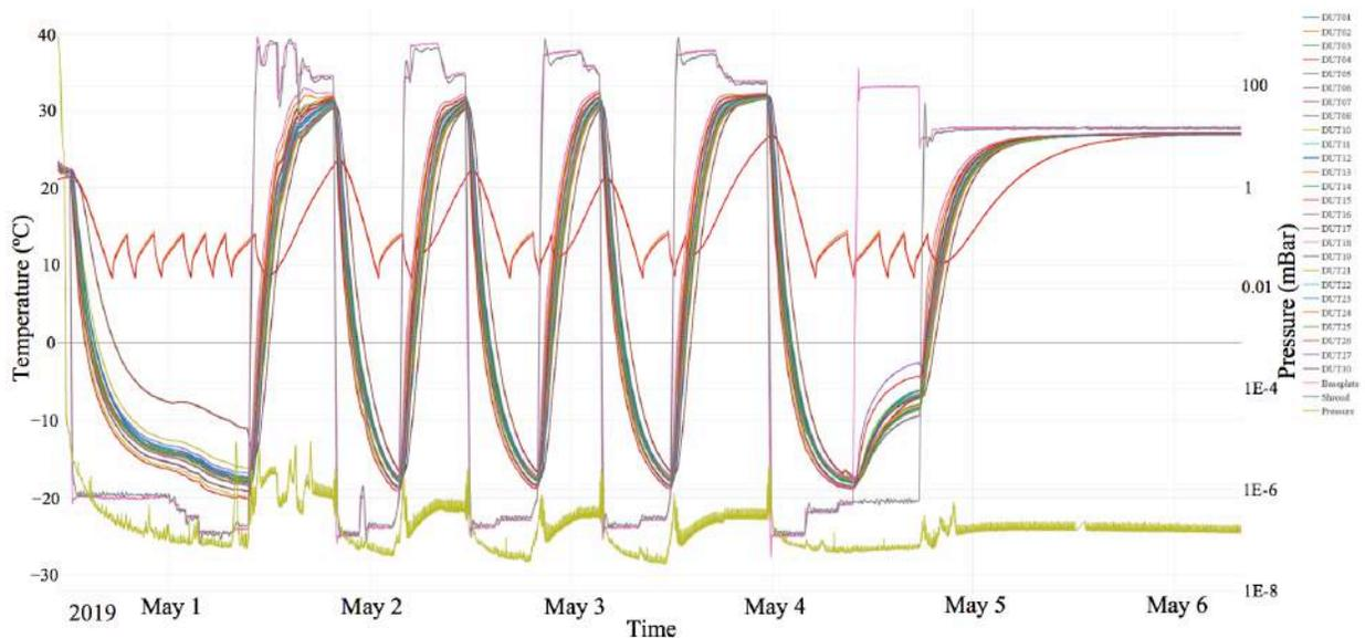
**Figure 13: Temperature and pressure values during the UPMSat-2 TVT campaign**
