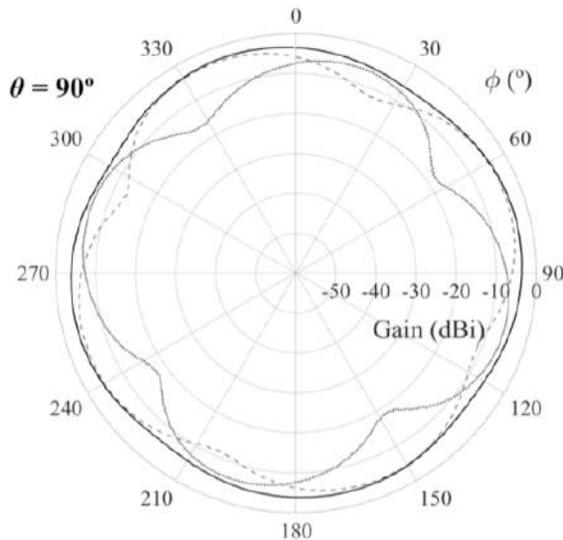
**Figure 8: UPMSat-2 antennae system radiation pattern (measured at INTA facilities). (- -) RHC polarization; (...) LHC polarization; and (-.-) total gain.**
