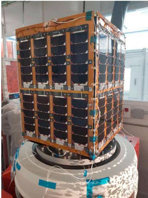
**Figure 5: UPMSat-2 lateral solar panels detail. Picture taken during the mechanical test campaign within the IDR/UPM institute facilities.**
