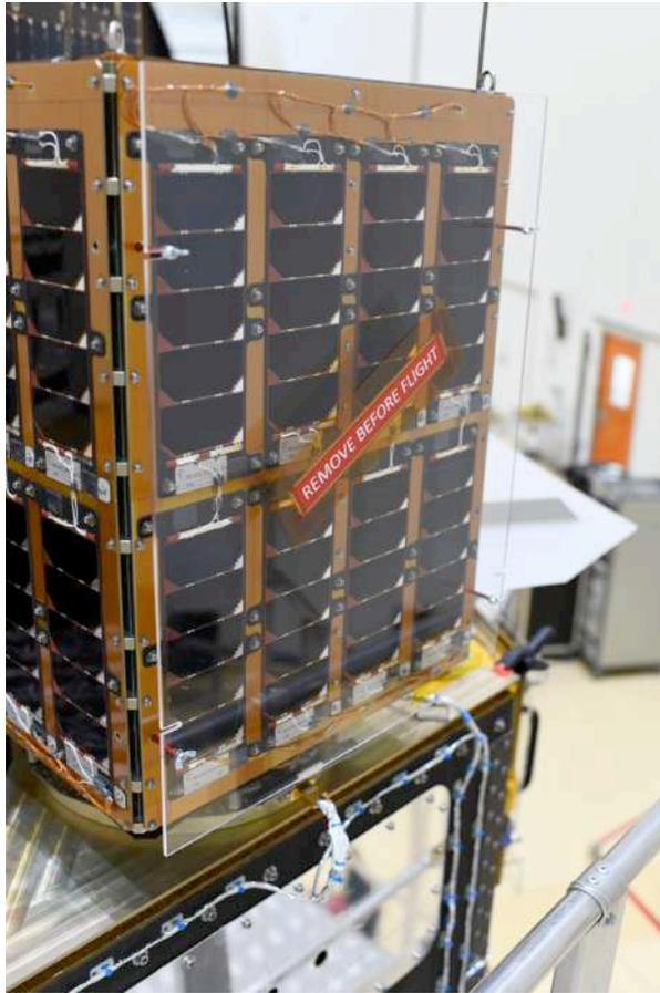
**Figure 17: UPMSat-2 fully integrated into a Tower Module of the Vega launcher SSMS dispenser.**
