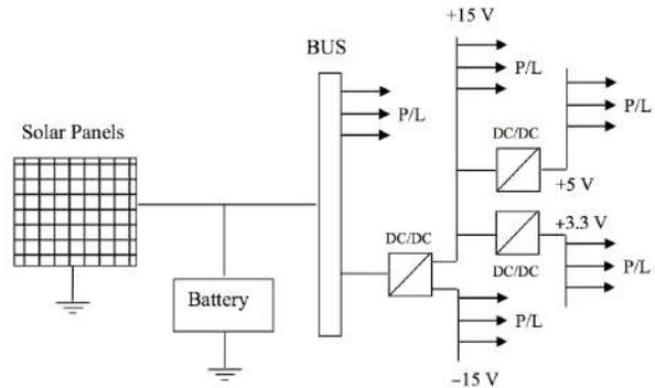
**Figure 2: Simplified sketch model of the UPMSat-2 power distribution system.**
